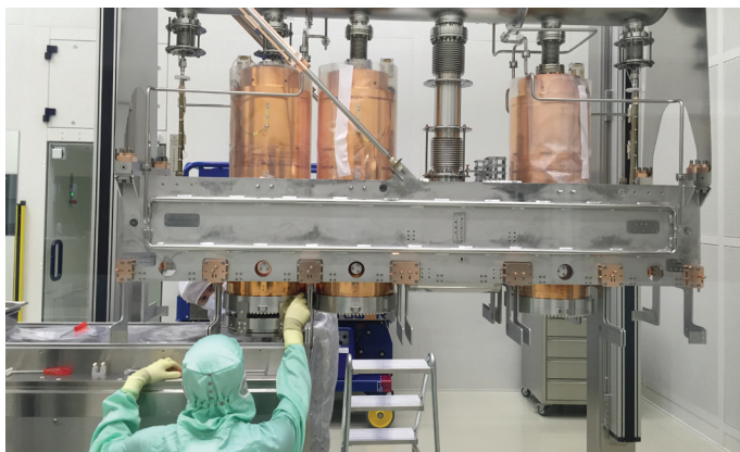
The assembly of the first superconducting cavities for HIE-ISOLDE began in a new clean room. (OPEN-PHO-ACCEL-2015 – 004)
