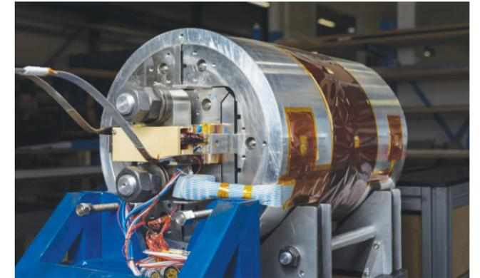
A record magnetic field of 16.2 Tesla was achieved using a flat coil, in the framework of the programme to develop more powerful magnets for future accelerators. (OPEN-PHO-ACCEL-2016-005-1)
