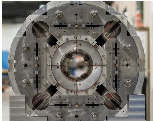
Structure for a "triplet" quadrupole magnet for the High-Luminosity LHC project. (OPEN-PHO-ACCEL-2015-014-2)
