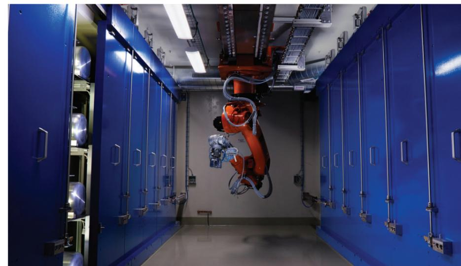
*A robotic sample changer at CERN’s MEDICIS and ISOLDE facilities allows different isotopes to be produced. (OPEN-PHO-EXP-2016-013-3)*
