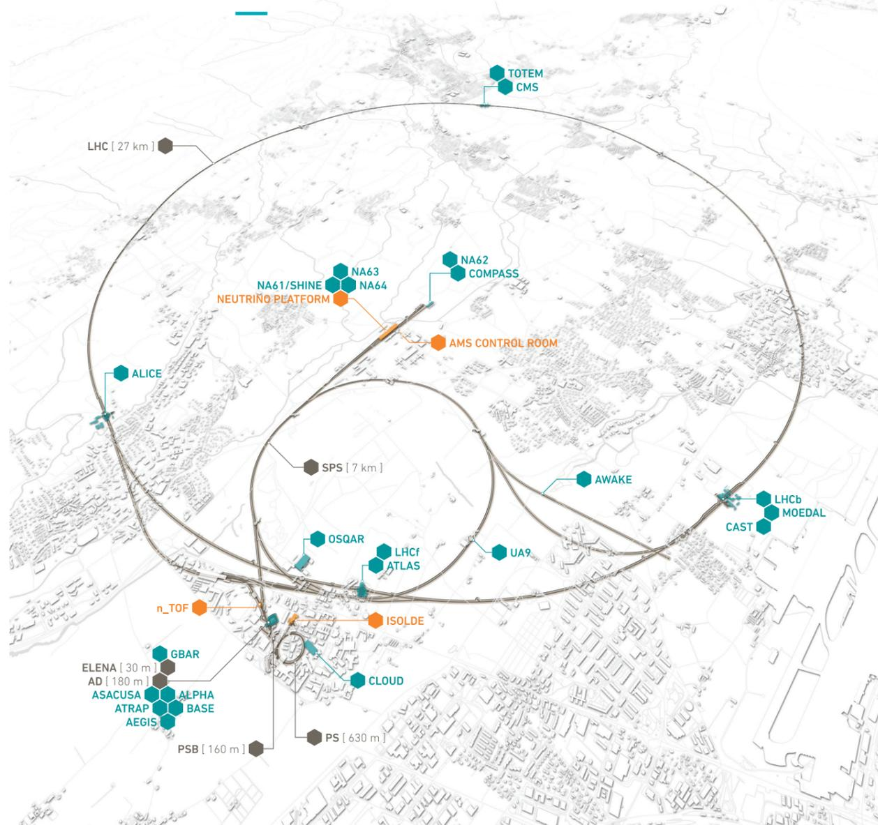
Focusing an energy of several teraelectronvolts (TeV) into a region measuring a millionth of a millionth of a millimetre across, the Large Hadron Collider (LHC) is the most powerful collider ever built, allowing physicists to explore uncharted subatomic territory. Measuring 27 km in circumference, the LHC produces tens of trillions of proton-proton collisions every day at the centre of four large detectors – ALICE, ATLAS, CMS and LHCb.
