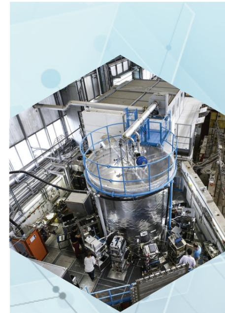
CLOUD comprises an ultra-clean and controlled environment into which beams of particles from the Proton Synchrotron are injected to simulate the seeding of cloud droplets. (CERN-EX-1310264-03)
