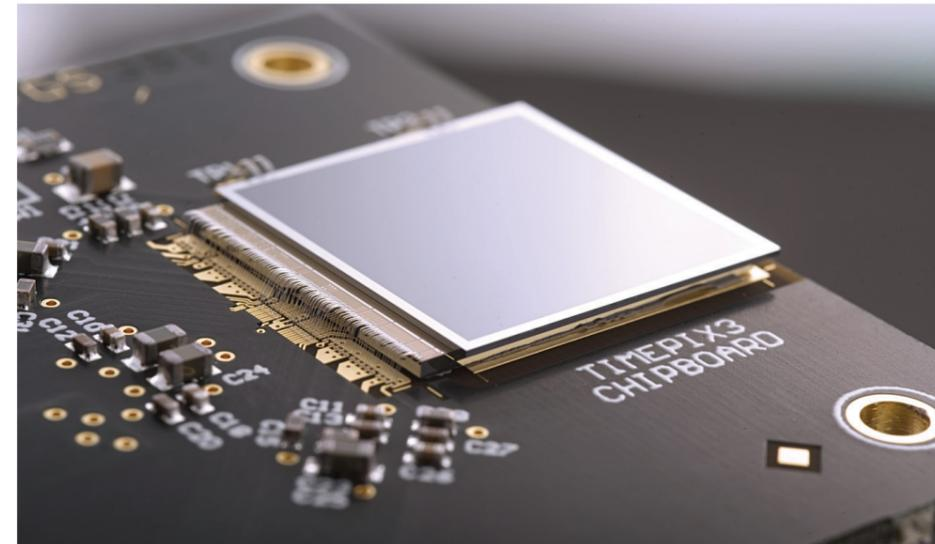
The Timepix3 chip is a multipurpose hybrid pixel detector developed in the framework of the Medipix collaborations, having applications in medical imaging, education, space dosimetry and material analysis. Originally developed for use in the LHC experiments, Medipix technologies are an outstanding example of how technology devised at CERN can create societal impact. (CERN-PHOTO-201702-048-4)
