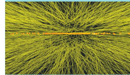
*A pile-up of several dozen collisions recorded in one bunch crossing by the CMS experiment in 2016. Each orange dot represents one collision. (CMS-PHO-EVENTS-2016-008-5)*
