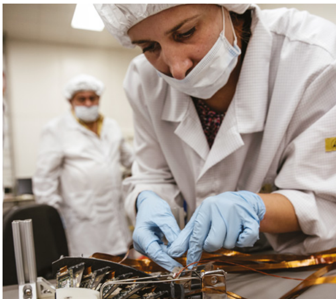
In 2016, CMS completed the assembly of its new pixel detector, which will allow improved reconstruction of charged particle tracks closer to the collision. (CERN-PHOTO-201609-239-6)
