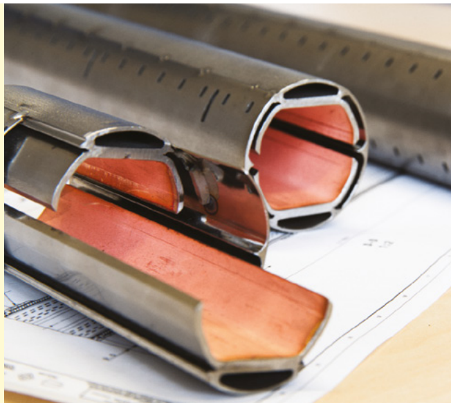
The first prototype for the FCC, a more efficient beam screen designed to disperse heat and maintain the ultra vacuum. (CERN-PHOTO-201604-074-2)
