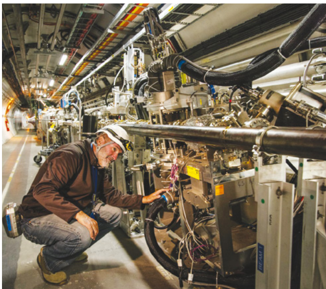
The TOTEM spokesperson in front of one of the experiment's detectors in the LHC tunnel, not far from the CMS detector. A special LHC run was provided for TOTEM and ATLAS/ALFA, with the beams as de-squeezed as possible. TOTEM upgraded its detectors in 2016. (CERN-PHOTO-201609-210-1)
