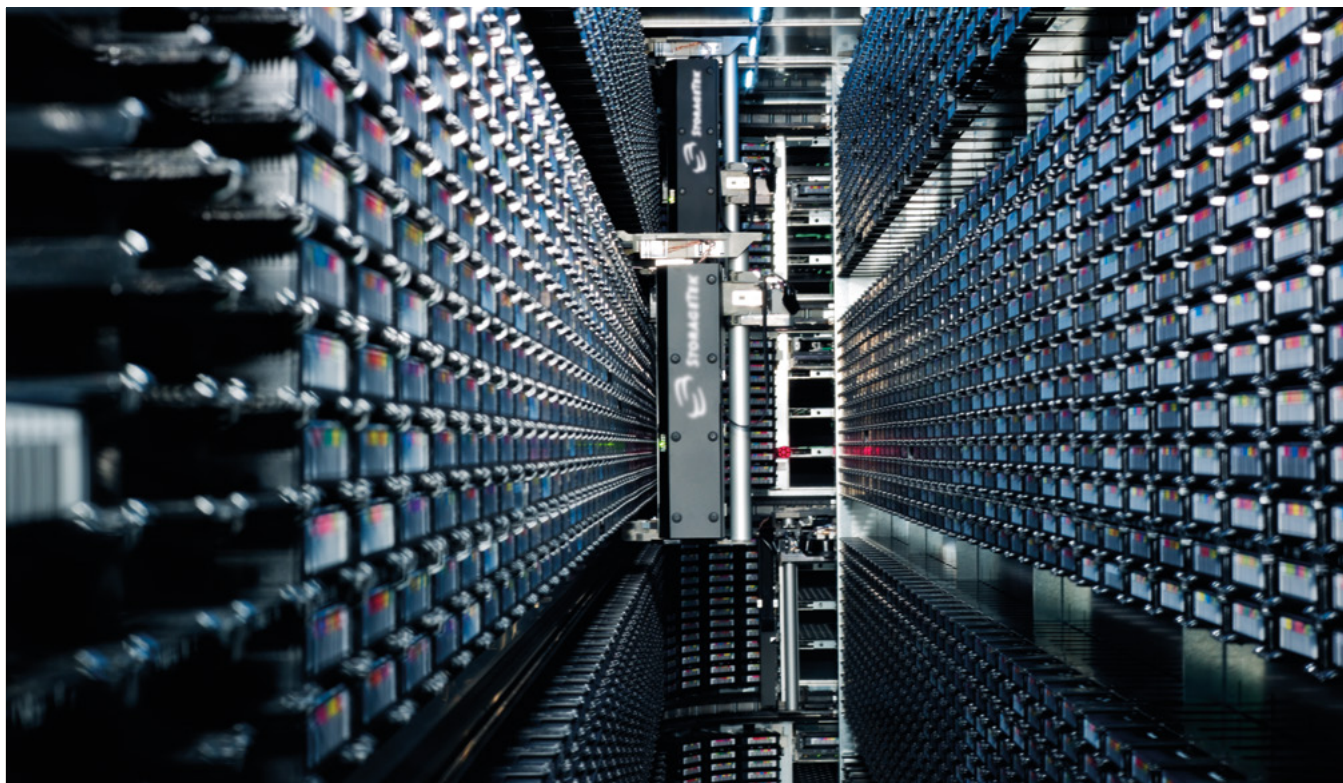
Magnetic tapes, retrieved by robotic arms, are used for long-term storage. (CERN-GE-0809016-01)
