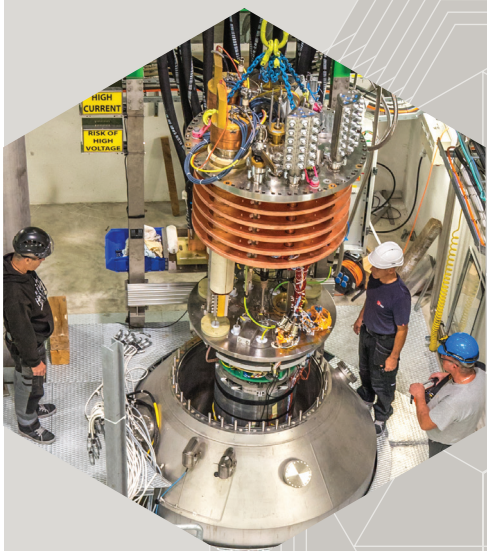
One of the short prototypes of the niobium-tin quadrupole magnets for the High-Luminosity LHC being inserted in the brand-new vertical test bench of the superconducting magnet test facility. (CERN-PHOTO-201708-191-20)
