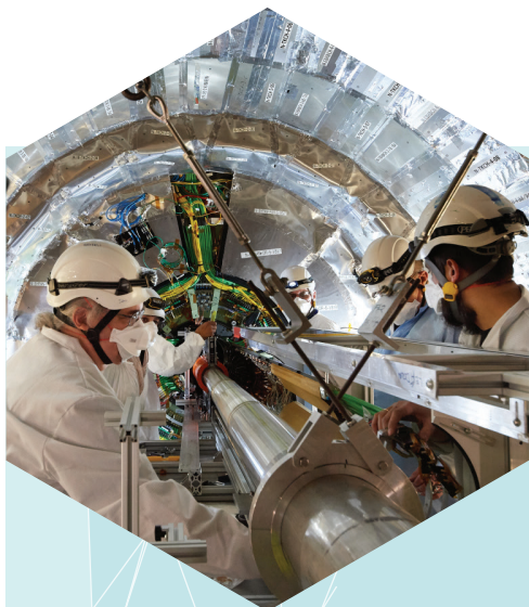
Open-heart surgery for CMS: the pixel tracker, the heart of the experiment, was replaced with a superior system before the 2017 LHC restart. (CERN-PHOTO-201703-062-43)
