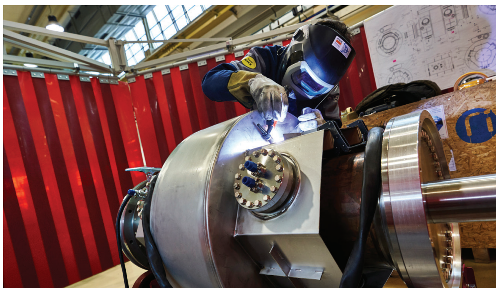
As part of the consolidation programme, a new accelerating cavity has been produced for the LHC, with performance levels higher than specification. (CERN-PHOTO-201803-084-1)
