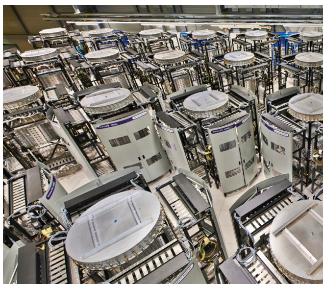
Installation of the new solid-state amplifier system developed for the SPS accelerating cavities. (CERN-PHOTO-201902-037-2)
