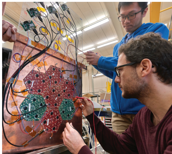
Prototype detector modules for the second phase of the upgrade of the CMS calorimeter. (CERN-PHOTO-201812-333-1)
