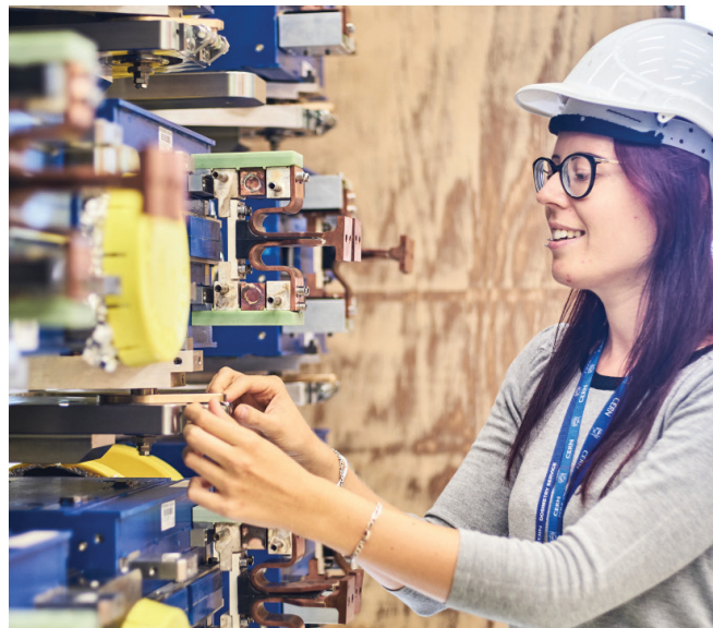
Mock-up assembly for the new injection system from the Linac4 to the PS Booster. This system is essential to achieve the required intensity and brightness of the proton beam in the PS Booster. (CERN-PHOTO-201708-201-7)
