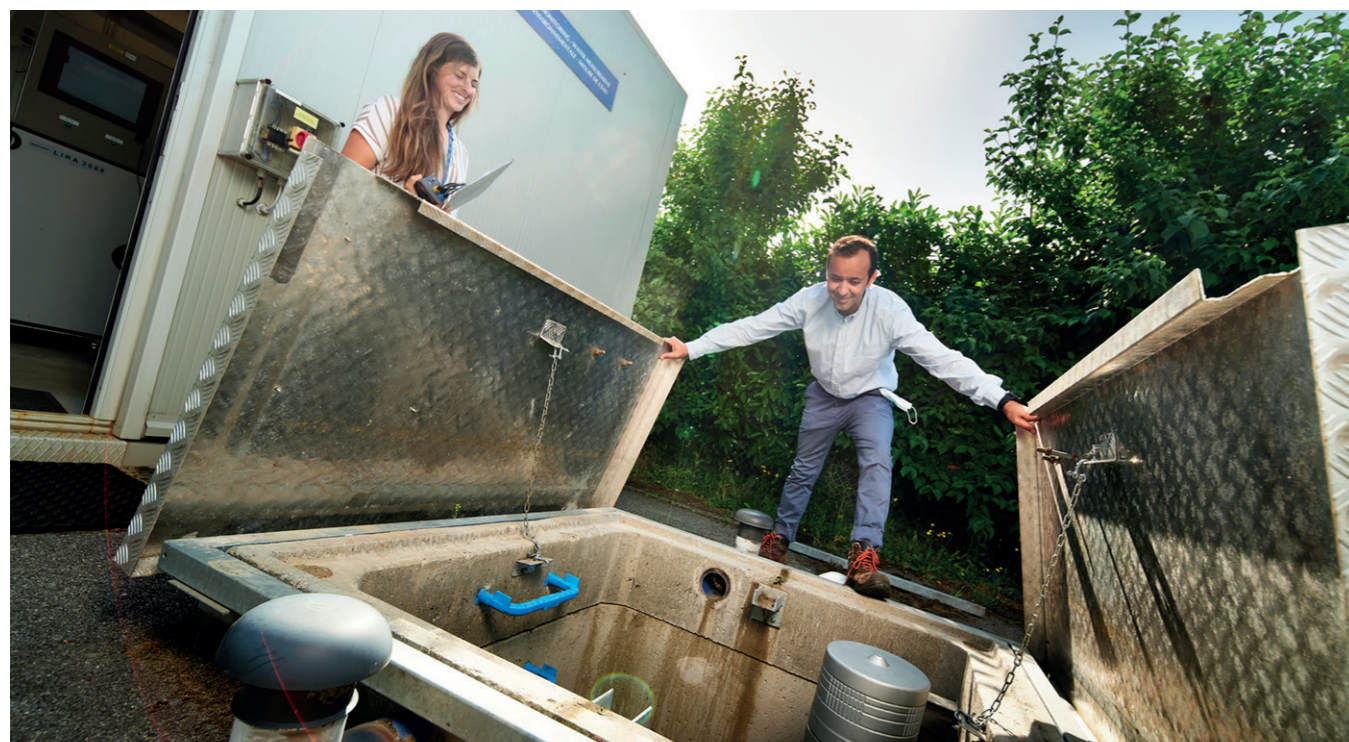
WATER MONITORING STATION with a hydrocarbon detection system at CERN's Meyrin site.
