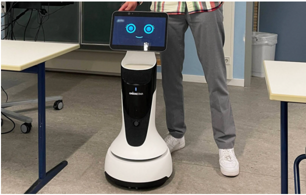
Fig. 1. This robot is used for testing and workshops in the school context. It can be remote-controlled by the ill child and has a screen on top to display the telepresence software.
