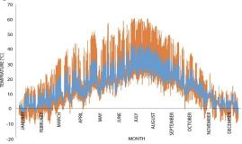
**Fig. 2.** Roof surface temperature comparison with (blue curve) and without (orange curve) the white coating over a year.
