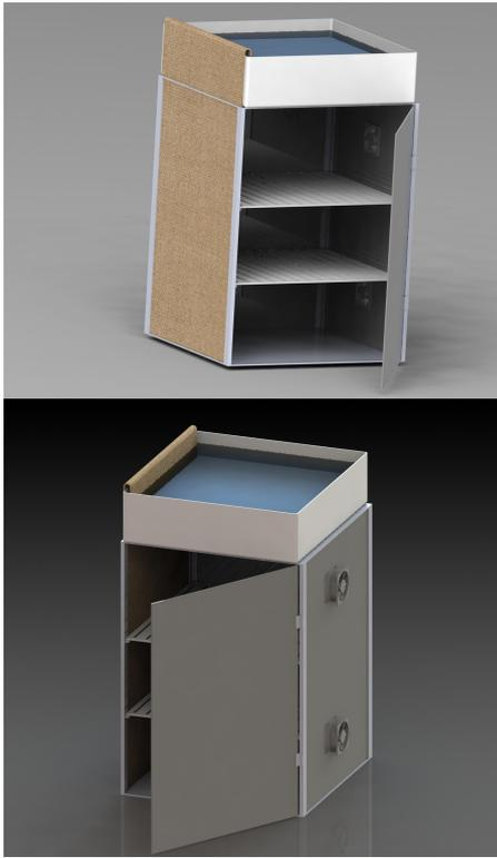
**Fig. 3.** CAD prototype of the evaporative cooler.
