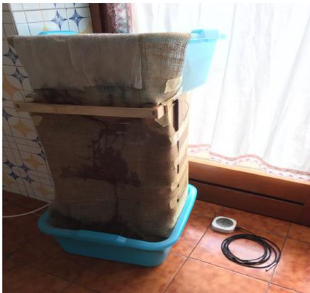
**Fig. 4.** Built prototype of the evaporative cooler.
