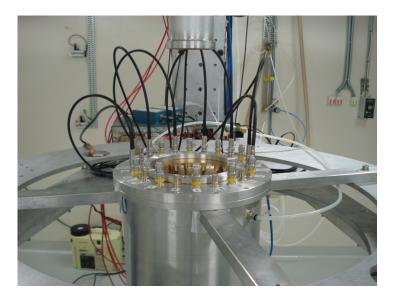
**Fig. 1:** A view of the chamber housing the samples and detectors, and the associated electronics placed in the neutron beam in EAR-2. The neutron beam arrives vertically from below and then continues in the vauum tube above the chamber and onto the beam dump a few meters later. Approximately 15-20 cm of air are present before and after the chamber.
