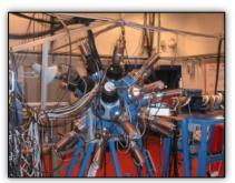
**Fig. 1:** (Color online) The Silicon Ring SiRi [16] and the  $\gamma$ -detector array CACTUS [15].
