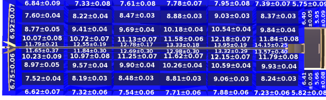
Fig. 10: Distribution of proportionality factor averaged over all long barrel counters of the first layer.
