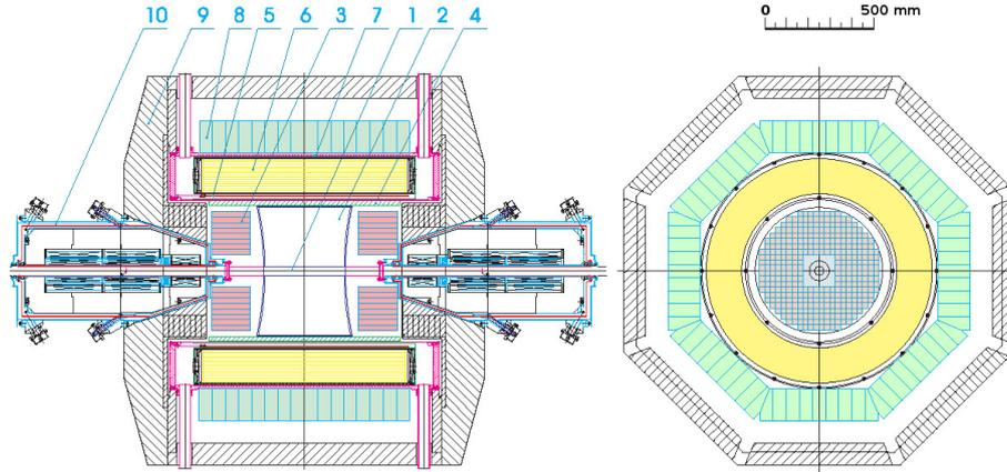
**Fig. 1:** The CMD-3 detector: 1 – beam pipe, 2 – drift chamber, 3 – BGO, calorimeter, 4 – Z-chamber, 5 – SC solenoid ( $0.13X_0$ ,  $1.3T$ ), 6 – LXe calorimeter, 7 – TOF system, 8 – CsI electromagnetic calorimeter, 9 – yoke, 10 – VEPP-2000 SC solenoids ( $13T$ ). The outer muon range system is not shown.
