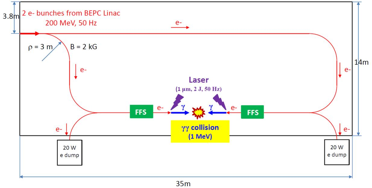
**Fig. 1:** Layout of a 1 MeV  $\gamma\gamma$  collider in an experimental hall at IHEP.
