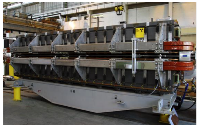
Figure 1: Picture of the PS combined function magnet unit.
