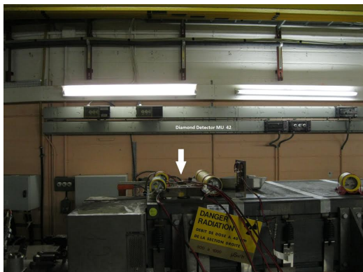
Figure 7: The white arrow in the picture indicates the position of the fast BLM on the top of main unit 42.
