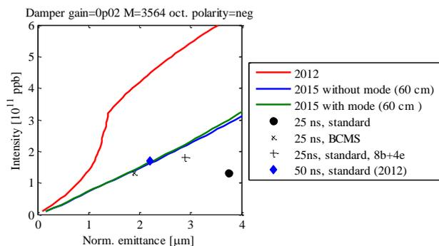
Figure 4: Impact of the 100 MHz mode of the 8 TCTP and 1 TCSG per beam on the stability limit as computed by the DELPHI code for a filled LHC with 25 ns bunch spacing, negative octupole polarity and  $\beta^*=60$  cm (in green), compared to the case without this “TCTP mode” (in blue) and to the 2012 case (in red). The beam is stable below the lines, unstable above the lines. The large difference between 2012 and 2015 is the result of the change of beam energy.
