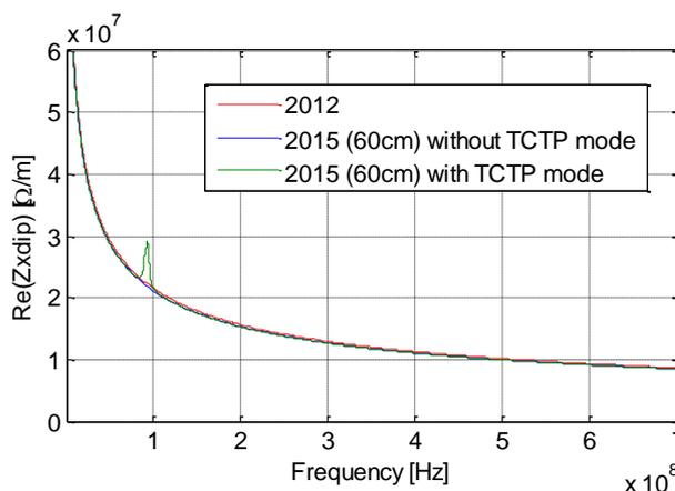
Figure 3: Impact of the 100 MHz mode of the 8 TCTP and 1 TCSG per beam on the real part of the horizontal impedance of the current LHC model for  $\beta^*=60$  cm (in green), compared to the case without this “TCTP mode” (in blue) and to the 2012 impedance model (in red).
