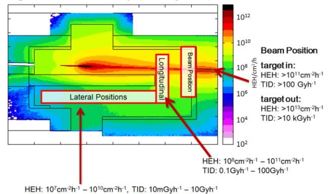
Figure 7: HEH flux (cm<sup>-2</sup>/h) inside the radiation zone.
