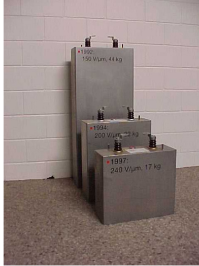
Fig. 8: A 2 mF 1800 V d.c. capacitor for input filters of TGV application. The sizes correspond to 150, 200, and 240 \text{ V}/\mu\text{m} in the dielectric.
