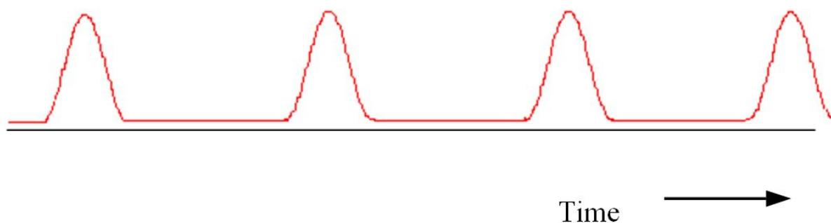
Fig. 3: Discontinuous acceleration cycles as used for ‘top-up’ injection; note that the delay between cycles is much in excess of the actual cycle time. Several strategies have been observed among top-up machines: at fixed interval (every  $x$  minutes or seconds) it is called  $dt$  (Diamond, APS); at fixed beam current decay (as soon as the  $I$  beam has decreased by  $x\%$ ) it is called  $dI$  (SLS, Elettra, Soleil, Bessy, Spring8, Petra).
