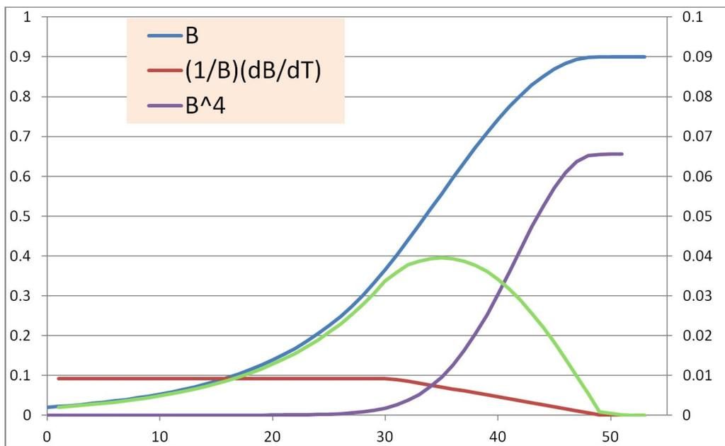
**Fig. 6:** A ‘custom specified’ field variation between injection and high energy (extraction) ( $B$ ), designed to provide a low gradient during and just after injection. Shown is the gradient ( $dB/dt$ ),  $B$  dot over  $B$  [ $(1/B)(dB/dt)$ ] and the function determining synchrotron radiation loss ( $B^4$ ).
