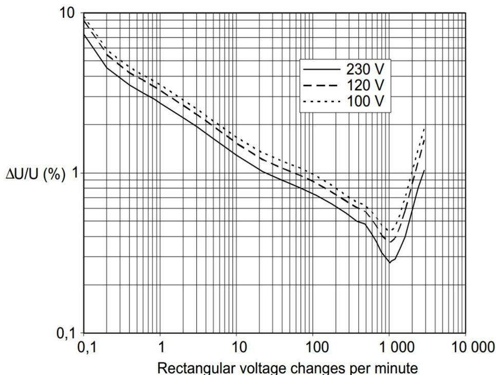
**Fig 13:** Curve of the maximum variation of supply voltage authorized on European networks. Note that two consecutive voltage changes (one positive and one negative) constitute one ‘cycle’, i.e., two voltage changes per second mean a 1 Hz fluctuation.
