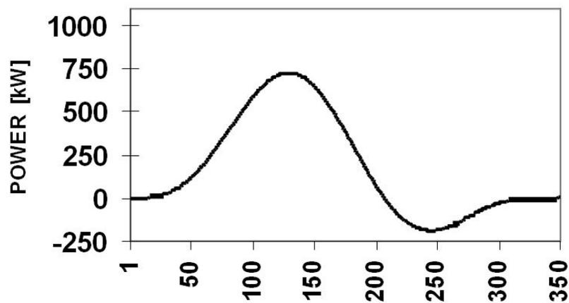
**Fig. 26:** Magnet power vs time (ms) in the SLS booster capacitive energy storage power supply system
