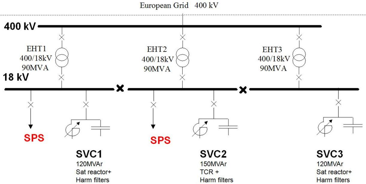
**Fig. 16:** Connection of filters using saturable reactors to the 18 kV feeder for the SPS magnet power supply system. The filters compensate for the inductive nature of the supply system and minimize phase swings that would otherwise occur, resulting from the power fluctuation during the acceleration and deceleration cycles.
