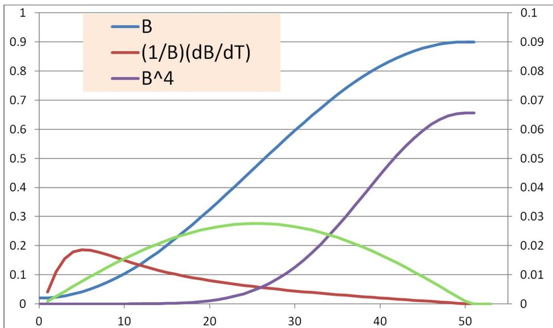
**Fig. 5:** A biased sine-wave field variation between injection and high energy (extraction) ( $B$ ). Also shown is the gradient ( $dB/dt$ ),  $B$  dot over  $B$  [ $(1/B)(dB/dt)$ ] and the function determining synchrotron radiation loss ( $B^4$ ).
