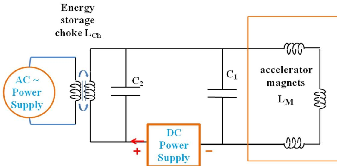
**Fig. 17:** Schematic diagram of a single-cell ‘White circuit’
