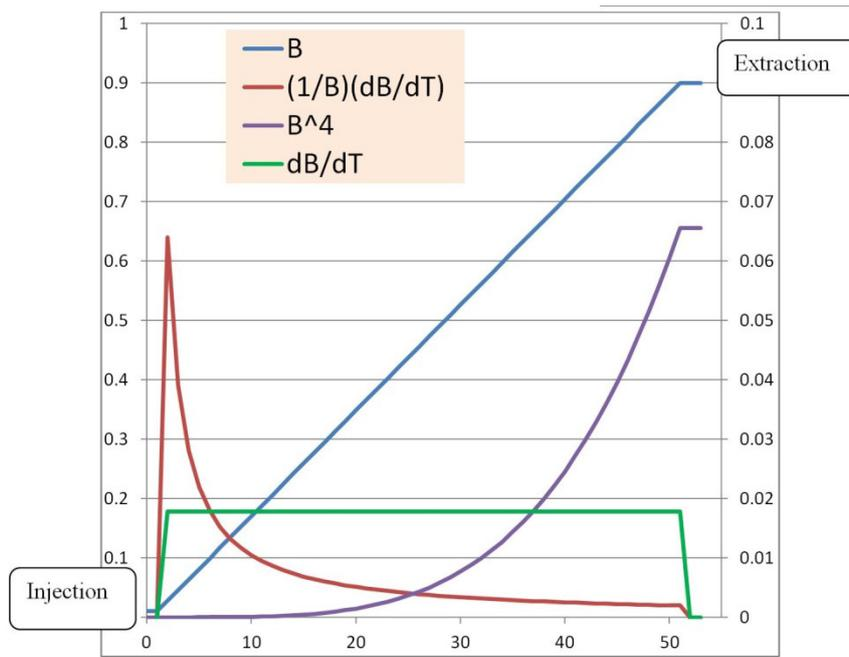
**Fig. 4:** A linear field ramp between injection and high energy (extraction) ( $B$ ). Also shown is the gradient ( $dB/dt$ ),  $B$  dot over  $B$  [ $(1/B)(dB/dt)$ ], and the function determining synchrotron radiation loss ( $B^4$ ).
