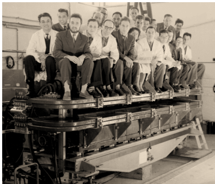
Fig. 6: Photograph from 1956 of the first PS magnet and members of the group who designed it. The CERN PS uses 100 of these magnets in the accelerator and one more on the surface for magnetic field measurements.
