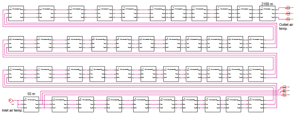
Fig. 6: The entire 2.1 km XTL tunnel with a total of 43 model components as a thermal circuit in the schematic of ANSYS SImplorer.
