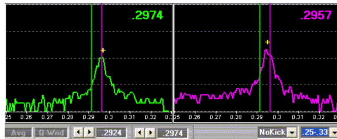
Fig. 20: Tune signal of a proton storage ring (HERA-p)
