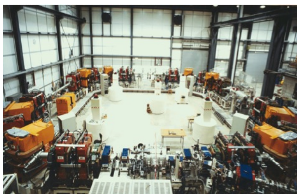
Fig. 12: TSR storage ring, Heidelberg, as a typical example of a separate-function strong focusing storage ring
