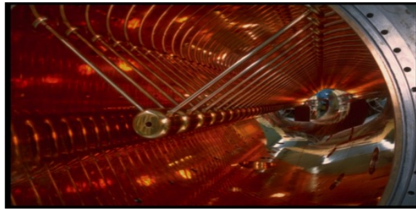
Fig. 9: Unilac at GSI, Darmstadt; clearly visible are the structure of the drift tubes and their increasing length as a function of the particle energy.
