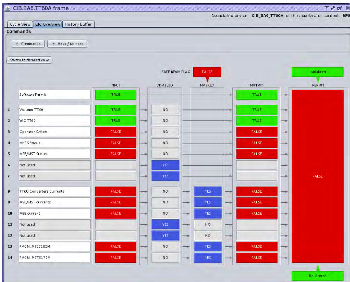
Fig. 21: Graphical user interface display of a beam interlock controller in TT60, which is the upstream part of LHC transfer line TI 2. Inputs 8–14 are maskable and can be disabled in case of intensity below the set-up beam flag . In this example, the set-up beam flag is false and the masks do not have an effect, i.e., in the column ‘matrix’ the masked inputs return false (red), despite the mask.
