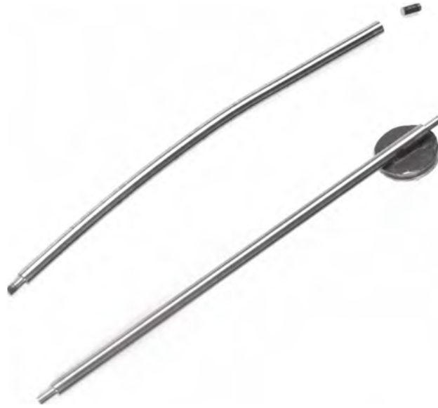
Fig. 2: Beryllium rods for first neutrino target installed at CERN-SPS. The unit on top was accidentally hit by an off-axis beam, leading to permanent bending and failure of the rod.
