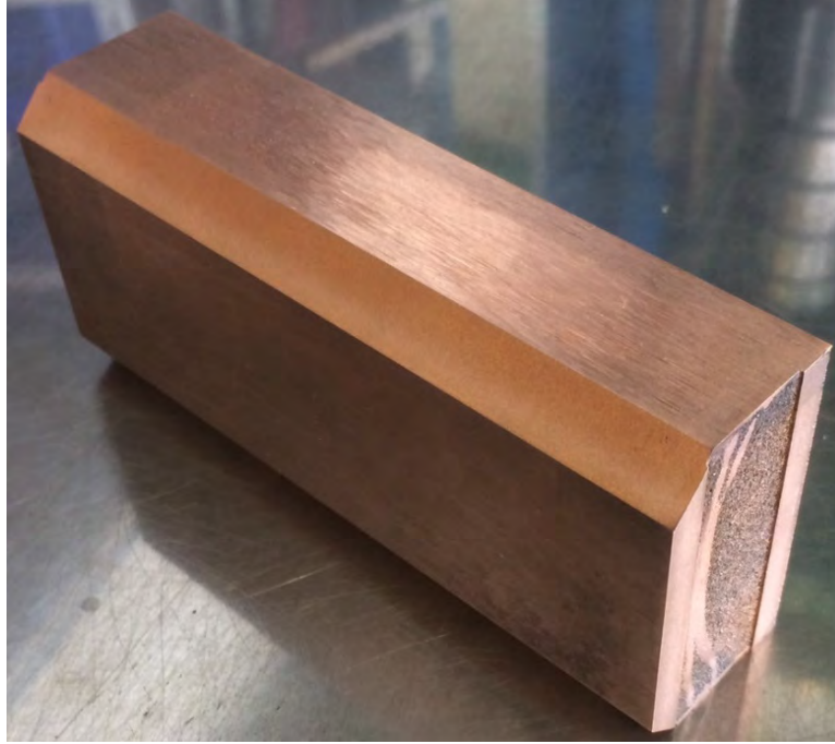
Fig. 48: CuCD block produced for a prototype jaw of HL-LHC secondary collimator [43]. Note the copper cladding on all functional surfaces.
