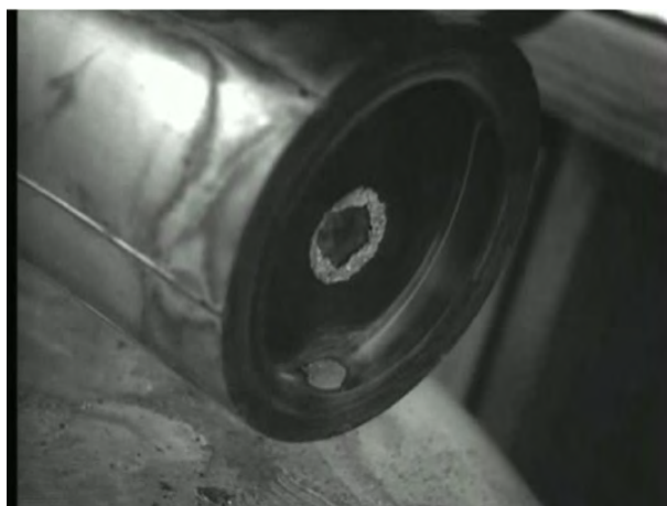
Fig. 10: A photograph of a failed target from the ISIS second target station. The tantalum cladding on the tungsten target failed. Figure reproduced from Ref. [16].
