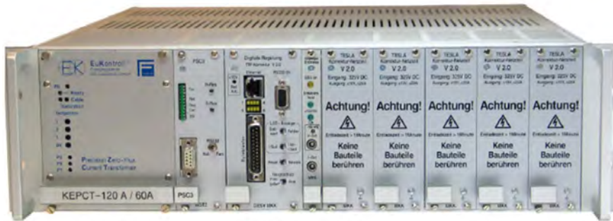
Fig. 5: Crate with five switched-mode power supplies, one of them being redundant (courtesy of J. Eckoldt, DESY)
