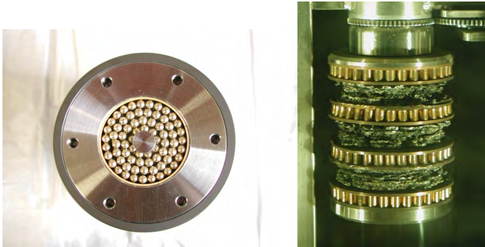
Fig. 9: Tevatron Run II antiproton production target. Left: Top view. Right: Target number 7 in 2007 with damaged Inconel discs and distorted copper cooling cylinders in between. Courtesy of A. Leveling and J. Morgan.
