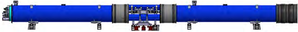
Fig. 37: Longitudinal integration of a TCLD collimator between two short 11 T dipoles. Courtesy of D. Ramos
