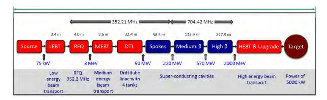
**Fig. 5:** Layout of the ESS accelerator: the source, low energy beam transport and RFQ are followed by the medium energy beam transport. The protons are accelerated by a normal-conducting linac, followed by three sections of superconducting cavities. In the high energy beam transport line the protons are transported to the target.
