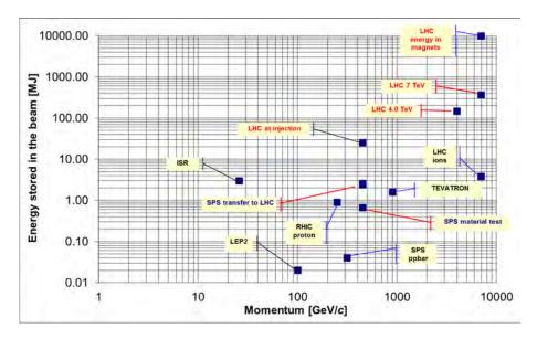
Fig. 2: Energy stored in the beams for different accelerators and the energy stored in the LHC magnet system
