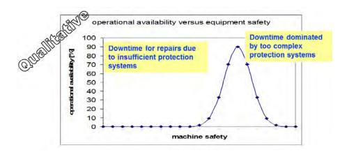
**Fig. 10:** Availability versus protection (qualitative graph). For too little protection, failures will lead to damage and reduce availability. For too much protection, the accelerator risks not being able to switch on and the availability is zero. There is some optimum in between.
