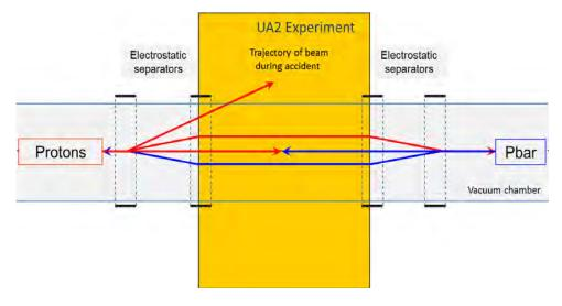
Fig. 14: Illustration of trajectories of proton and antiproton beams for collisions, during injection and during the accident.
