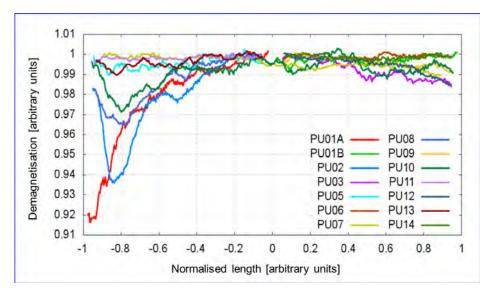
Fig. 4: Demagnetization of undulators at the PETRA storage ring from [13]
