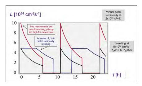
Fig. 9: Luminosity levelling at HL-LHC
