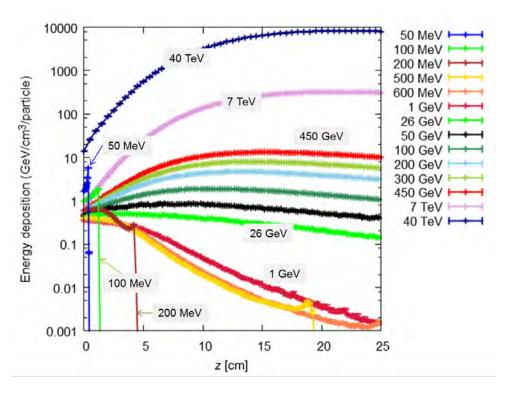
Fig. 11: Proton energy deposition for different energies for the impact of protons on copper [21]
