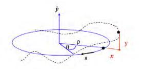
Fig. 3: The trajectory coordinates are given with respect to the Frenet–Serret frame, which rotates with the ideal particle around the accelerator. The ideal particle has design momentum  $p_0 = m_0 \gamma v$ . It has coordinates x = 0, y = 0 for a certain longitudinal location s lying on the design orbit.
