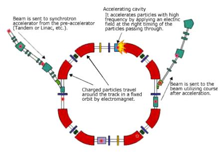
Fig. 1: Typical layout of synchrotron
