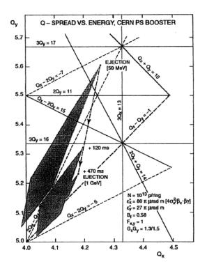
**Fig. 14:** Tune spread due to the space-charge effect for high-intensity beams in the CERN PS Booster. Injection energy, 50 MeV; maximum extraction energy towards the CERN PS, 1.4 GeV.
