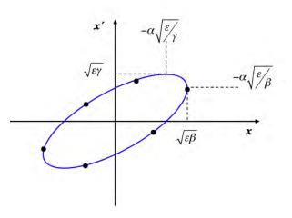
Fig. 5: The trajectory of a particle in phase space x, x', turn after turn, is an ellipse. The orientation and shape is defined by the focusing properties of the lattice, whereas the area of the ellipse is an intrinsic property of the beam.
