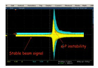
**Fig. 12:** Beam position measurement at a beam position monitor turn-by-turn. During the instability, the trajectory amplitude grows exponentially until the beam loses intensity and stabilizes itself.
