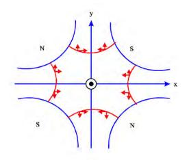
**Fig. 2:** A schematic cross-section of a quadrupole magnet. The red arrows indicate the direction of the force on the particle. A quadrupole that is focusing in the horizontal plane is defocusing in the vertical plane.
