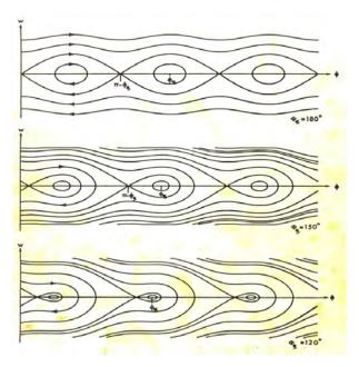
**Fig. 9:** The buckets around the ring shrink during acceleration when the synchronous phase is moved towards  $90^{\circ}$  (Courtesy of F. Tecker.)
