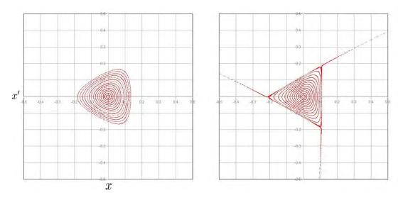
Fig. 11: The trajectories in phase space x, x' with sextuple fields in the ring. The size of the stable area within the triangle is a function of the distance of the tune from the third-order resonance.
