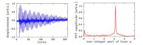
**Fig. 4:** Turn-by-turn oscillation recorded at a beam position monitor after a one-turn excitation with a kicker magnet on the left side. The fast Fourier transform spectrum of this oscillation on the right side. The amplitude peak in the spectrum indicates the tune of the oscillation.
