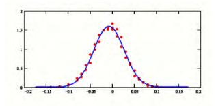
Fig. 6: Transverse profile measurements of a particle beam (red dots), using a wire scanner, and Gaussian fit (blue line).
