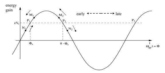
Fig. 7: The principle of phase stability (Courtesy of F. Tecker)
