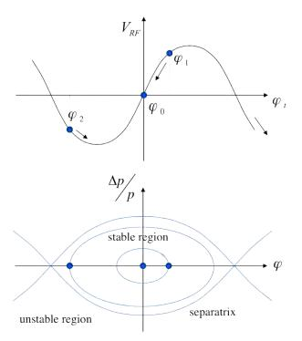
**Fig. 8:** The longitudinal motion in the upper plot follows the trajectory in phase-space in the lower plot. The separatrix defines the limit of stable motion (Courtesy of F. Tecker.)
