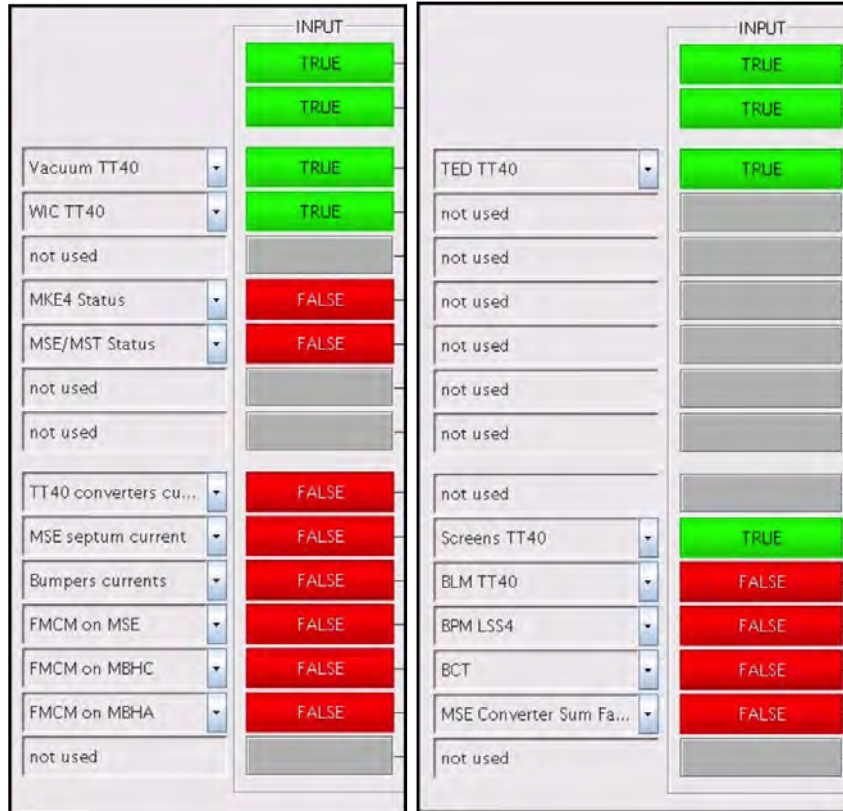
Fig. 20: Graphical user interface displays of two beam interlock controllers in TT40, the upstream part of transfer line TI 8. The vacuum system, the warm magnet interlock system (WIC), the extraction kicker MKE4 state, the septa MSE and MST states, the TT40 power supply currents, the septa currents, the orbit bump corrector magnet currents, the fast magnet current change monitors (FMCM), which survey fast changes in case of failures instead of absolute current values, the optical transition radiation (OTR) screen positions, the beam loss monitors (BLM) and the extraction orbit with BPM LSS4 are all input to these interlock controllers.
