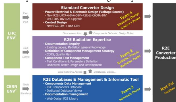
Figure 5: The radiation tolerant design of the power converters is based along three teams: the converter design, radiation test and management/documentation.
