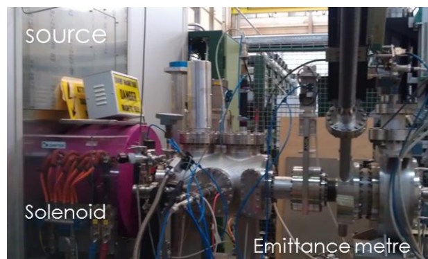
Figure 2: Set-up for emittance measurements at 45 keV.
