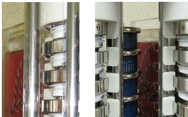
Figure 11: GTO stacks before LS1 (left) and after LS1 (right) with additional high-voltage insulation.
