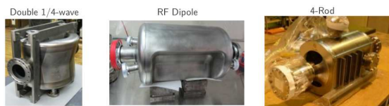
Figure 1: Prototype Niobium cavities of the DQW, RFD and the 4-Rod respectively [5].
