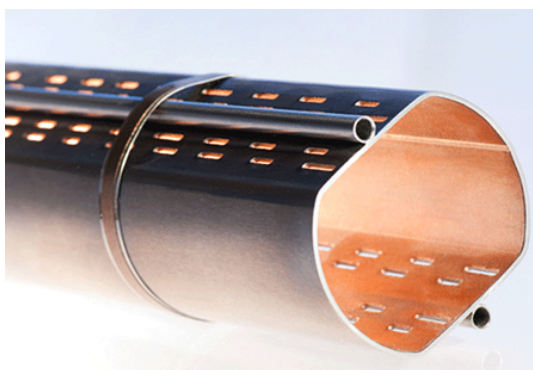
Figure 2: Beam screen with the associated cooling tubes
