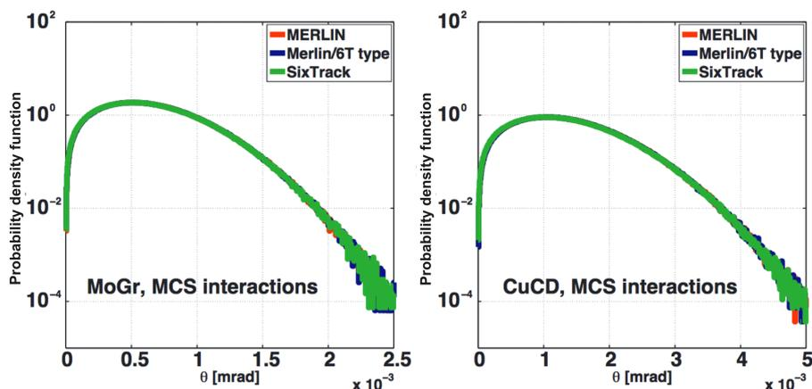
**Fig. 3:** Distribution of polar angle  $\theta$  for multiple Coulomb scattering and ionisation events in MoGr (left) and CuCD (right) block. Comparison of simulation results using “MERLIN-method”, “MERLIN-6T-method”.
