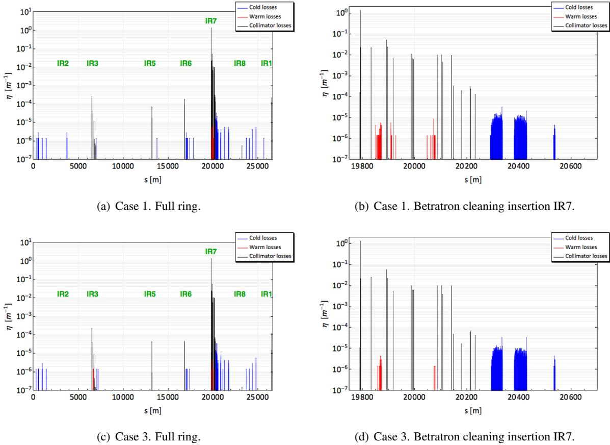
**Fig. 5:** Beam loss patterns at 7 TeV in the nominal LHC machine for Beam 1 horizontal halo, simulated by SixTrack. In blue, the losses in the superconductive magnets (cold losses), in red those in the normal-conductive magnets (warm losses) and in black the losses in the collimators.
