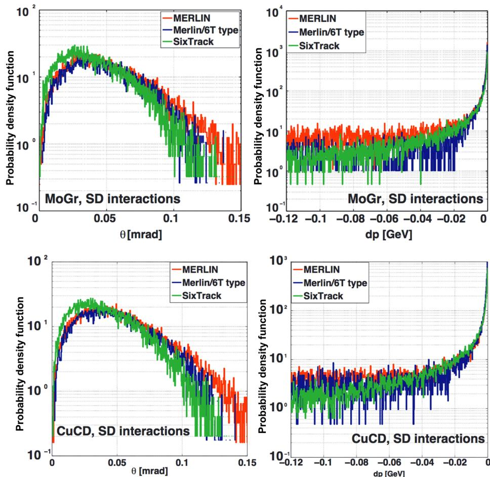
**Fig. 2:** Distribution of polar angle  $\theta$  (left) and energy loss  $dp$  (right) for single diffractive events in MoGr (top) and CuCD (bottom) block. Comparison of simulation results using “MERLIN-method”, “MERLIN-6T-method” and SixTrack.
