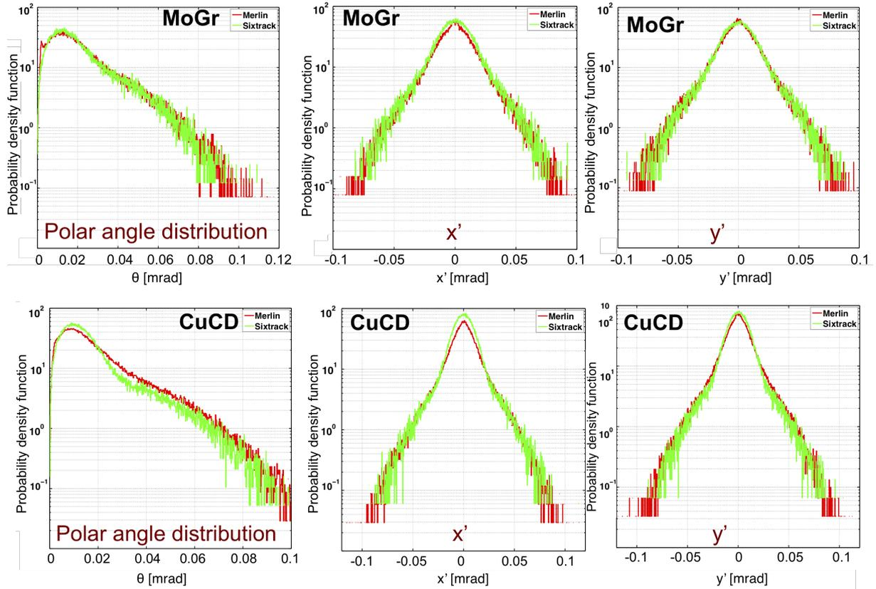
**Fig. 4:** Polar angle distribution (left) and distributions in  $x'$  (center) and  $y'$  (right) after 1 cm of CuCD (bottom) and in 1 cm of MoGr (up) of total elastic scattering, comparing MERLIN and SixTrack.
