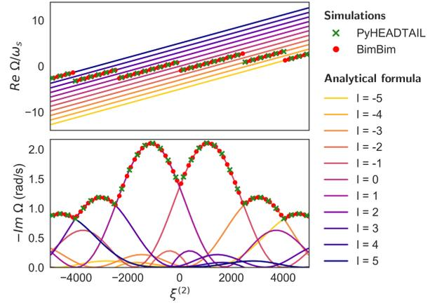
Figure 2: Real (top) and imaginary (bottom) coherent frequency shifts as a function of  $\xi^{(2)}$  at fixed  $\xi^{(1)}$  for an airbag model.
