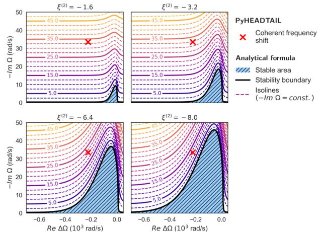
Figure 3: Stability boundary diagrams for four different values of  $\xi^{(2)}$  increasing in absolute value from top left to bottom right.
