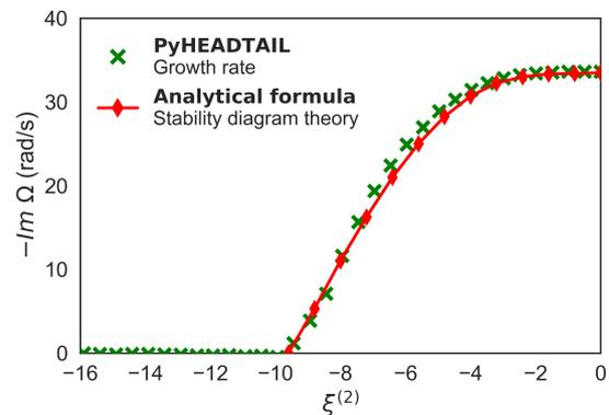
Figure 4: Stabilization of the head-tail mode zero vs.  $\xi^{(2)}$  for a Gaussian beam. PYHEADTAIL simulations (green crosses) are shown together with analytical predictions calculated by means of stability diagram theory (red diamonds).
