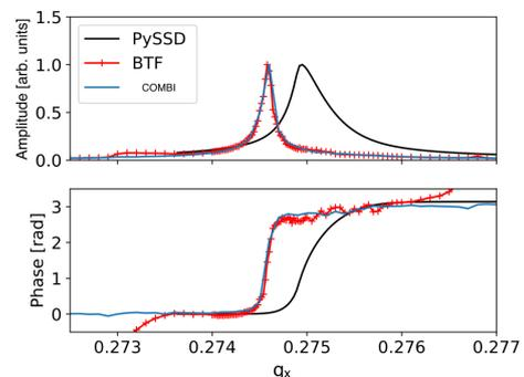
Figure 9: Measured BTF response at flat top energy (red line) compared to simulated BTF response (the blue line) including in the model the impedance and an octupole current of 546 A (as during the measurements). The analytical case without impedance is the black line.
