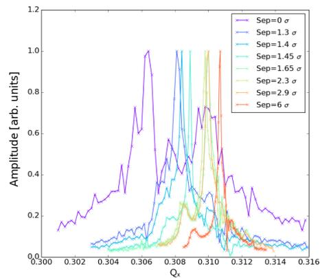
Figure 11: Measured BTF amplitude responses with head-on collisions in IP1 and IP5 for different offsets at the IPs.
