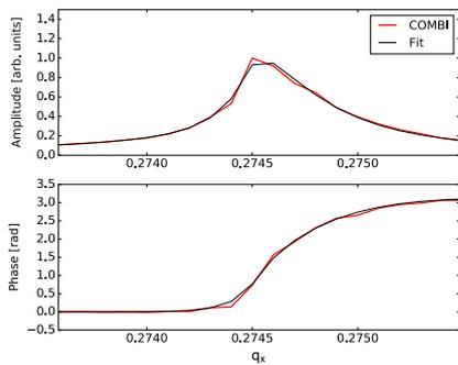
Figure 2: Amplitude and phase BTF responses simulated by using the COMBI code (red line) in the presence of linear detuning with amplitude. The black line represents the results of the parametric fit. The same tune spread has been applied for both cases and, as expected, the fit gives a tune spread factor close to 1 ( $p_1 = 1.02$ ).
