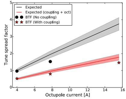
(b) Tune spread factors measured in the vertical plane.
