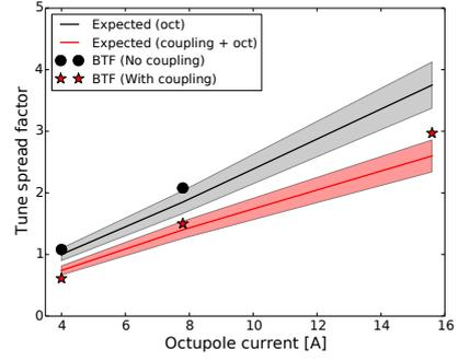
(a) Tune spread factors measured in the horizontal plane.
