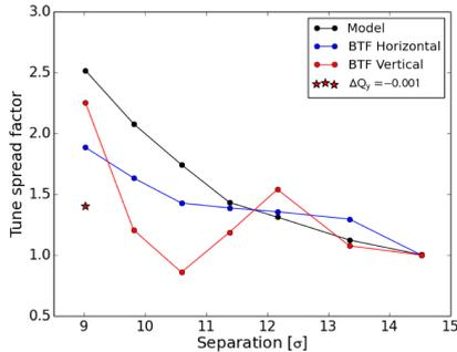
Figure 10: Measured tune spread factor as a function of the long range encounter separation at the interaction points in units of the rms beam size. Measurements were acquired at the end of the betatron squeeze. The red star represents the measured tune spread in the vertical plane with a reduced tune of  $\Delta Q_y = -0.001$ .
