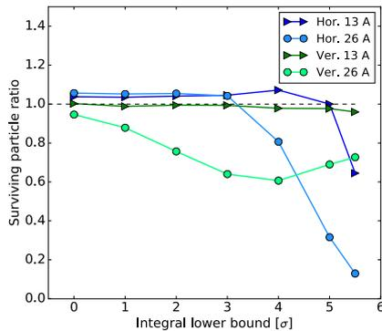
Figure 5: Surviving particle ratio as a function of the integral lower bound. The dark blue line with dark blue triangles and the light blue dotted line represent the horizontal plane for an octupole current of 13 A and 26 A respectively. The dark green line with dark green triangles and the light green dotted line represent the vertical plane for an octupole current of 13 A and 26 A respectively.
