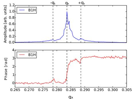
Figure 1: Example of a BTF measurement: amplitude and phase response for B1 in the horizontal plane at the LHC injection energy. Synchrotron sidebands are visible in the amplitude, with the corresponding phase jumps at  $q_x \pm Q_s$  (where  $Q_s = 5 \times 10^{-3}$ ).
