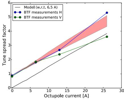
Figure 4: Measured tune spread factors as a function of the octupole current at injection energy in the horizontal (the blue dots) and in the vertical (the green dots) planes. The solid black line represents the factors expected from the model for a current  $I_{oct} = 6.5$  A. The red shadow represent the model expectations including the initial non-zero tune spread corresponding to  $\approx 5.5$  A with an uncertainty of  $\pm 10\%$  on the measured emittance.
