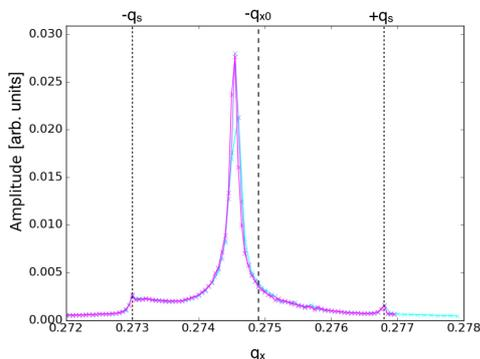
Figure 7: Various horizontal BTF acquisitions for Beam 1 at flat top energy. The chromaticity was reduced to 2.5 units during the measurements. The black dashed lines corresponds to synchrotron sidebands at  $q_{x0} \pm q_s$  with  $q_{x0}$  the incoherent bare tune in the horizontal plane.
