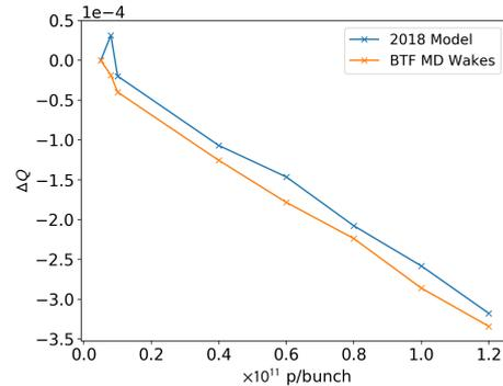
Figure 8: Coherent tune shifts as a function of bunch intensity. The tune shifts have been evaluated from the simulated BTF response including the 2018 wake field model (light blue line) and the wake field evaluated from the collimator settings as during the MD (orange line).
