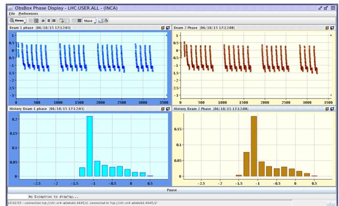
Figure 12: Screenshot of the graphical user interface (by G. H. Hemelsoet) of the bunch-by-bunch phase measurement with the phase-module. Clear e-cloud signatures along the bunch trains can be observed at the top plots, both for Beam 1 (left) and Beam 2 (right).
