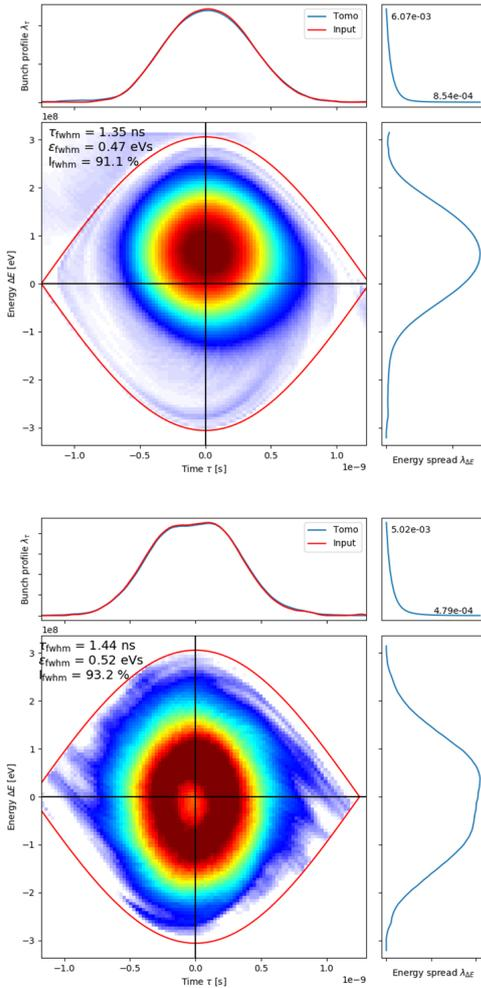
Figure 4: Tomographic reconstruction of a bunch in the LHC. Top: at the moment of injection. Bottom: 30 minutes later. A hole in the center of the longitudinal phase-space is generated due to the large energy error, and survived until the beginning of the ramp.
