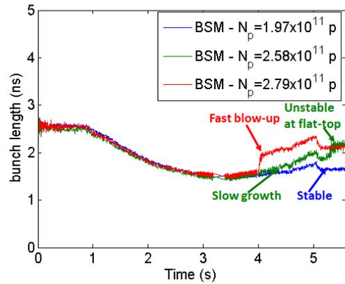
Figure 5: Bunch length evolution at the SPS in double harmonic operation (bunch shortening mode) for different intensities. Blue trace: stable bunch. Green trace: slow instability manifests with slow emittance blow-up during the ramp. Red trace: fast instability indicated by a sudden increase of the bunch length (microwave instability) [5].
