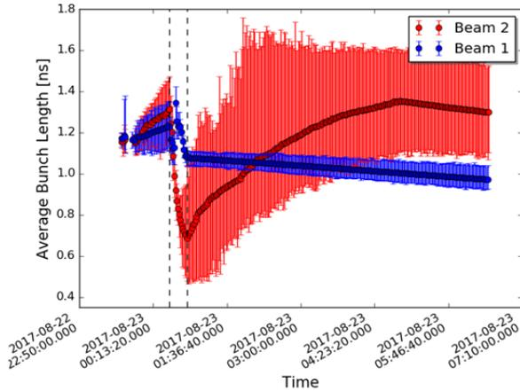
Figure 10: Example of the average bunch length evolution during a nominal LHC cycle. Continuous reduction of the average bunch length of Beam 2 during the ramp (marked by the two vertical dotted lines), since controlled longitudinal emittance blow-up was not applied. The instability threshold was reached and many bunches became unstable, indicated by the large bunch length spread.
