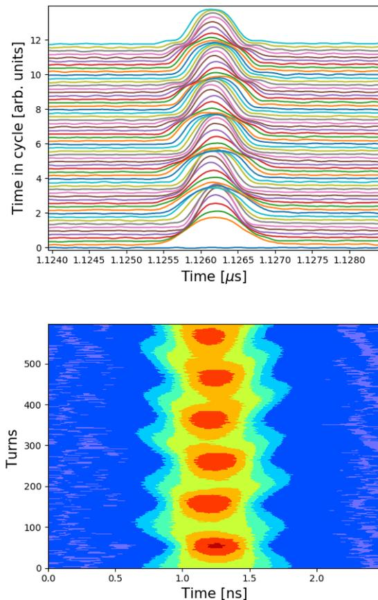
Figure 1: Two common illustrations of longitudinal bunch profile measurements at the LHC injection ( $V_{RF} = 6$  MV). Top: "mountain range" plot. Bottom: "waterfall" plot. The quadrupole oscillations of the bunch are clearly visible, initiated by an RF voltage mismatch.
