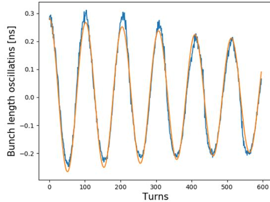
Figure 3: Bunch length oscillations at the LHC injection with  $V_{RF} = 6$  MV. The synchrotron frequency  $f_s = 54.9$  Hz and damping time of  $\tau_d = 0.15$  s were obtained after applying a sinusoidal fit (orange curve). The revolution period is  $T_{rev} = 88.9 \mu\text{s}$ .
