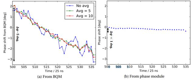
Figure 11: Bunch-by-bunch phase shift computed from bunch positions measured by the BQM (left) and by the phase-module (right). The larger phase shifts in BQM (a) are due to beam loading. In both cases the one-turn feedback is off [9].
