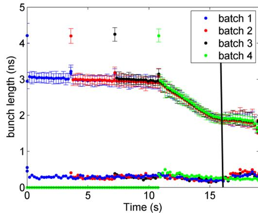
Figure 6: Average bunch length evolution along a nominal LHC proton cycle in the SPS. Different colours correspond to different batches of 72 bunches. The dots on the bottom show the bunch length spread within each batch. The black solid line corresponds to the onset of the instability.
