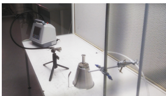
Figure 3: Particle size measurement set-up.
