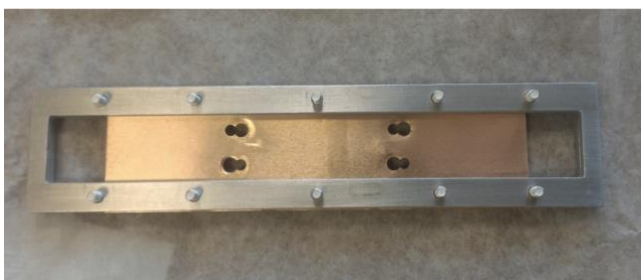
Figure 5: Slab placed in the frame for the deposition.
