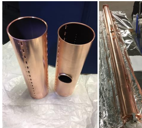
Figure 18: Left, segments of laser treated tube before their assembly at CERN, right assembled laser treated tubes to form a beam screen before its insertion into COLDEX [18].
