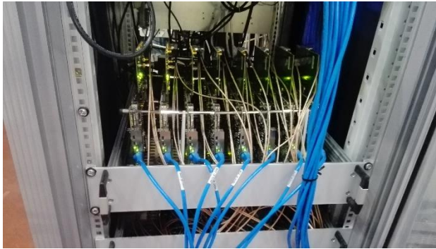
Figure 5: DAFNE 3+L data acquisition system based on 8 FPGA based boards working in parallel.
