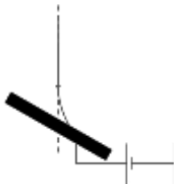
Figure 4: Deviation from straight line for electrons impinging on a sample with a negative bias voltage.
