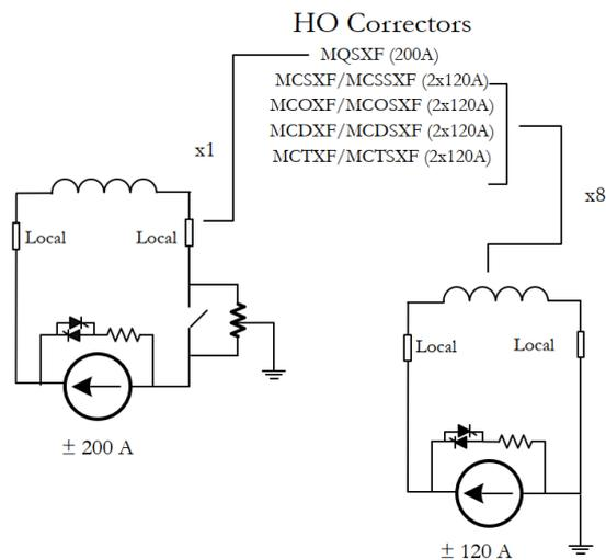
Figure 6-7: Superferric, higher order correctors' circuit layout.
