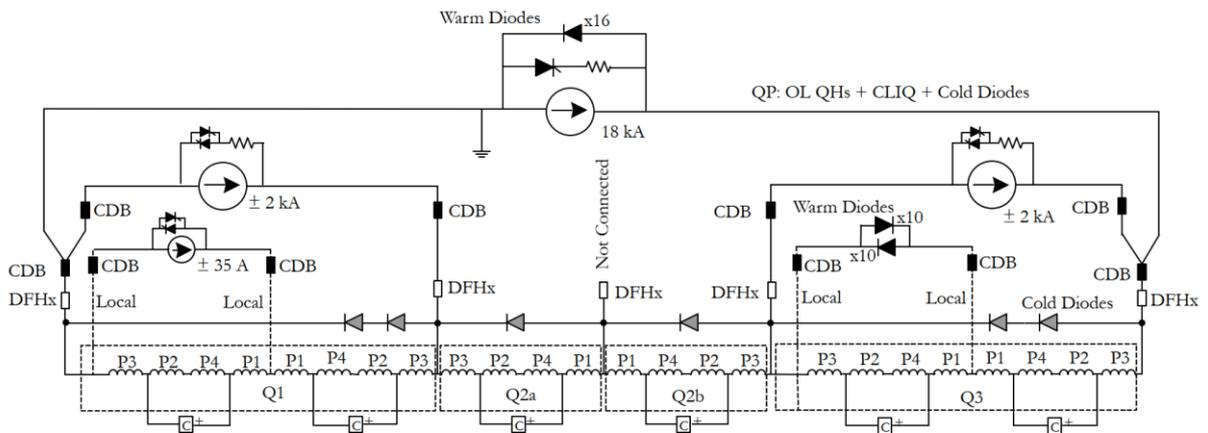
Figure 6-4: Circuit layout of the HL-LHC inner triplet.
