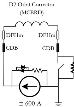
Figure 6-10: D2 correctors' circuit layout.
