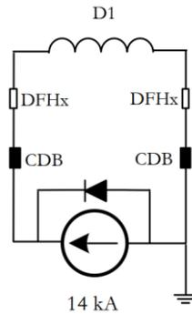
Figure 6-8: D1 magnet circuit layout.
