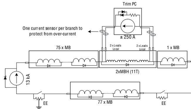
Figure 6-13: Circuit layout of the 11T trim circuit.
