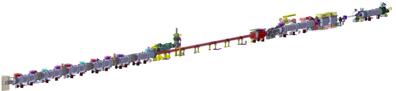
Figure 15-1: 3D integration model of the high-luminosity insertion regions of IR1 and IR5 of the HL-LHC machine. From left to right: Q1, Q2, Q3, D1, Corrector Package, DFX, DFM, TAXN and collimators, D2, 2 Crab Cavities cryo modules, Q4.
