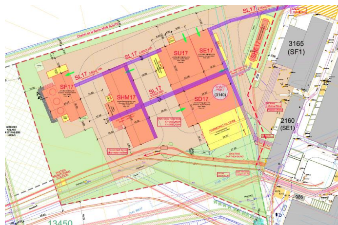
Figure 15-8: The LHC Point 1 with the new HL-LHC surface buildings in orange. Simple concrete slabs are highlighted in yellow.
