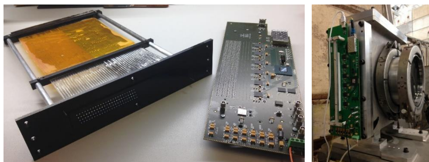
Fig. 4-37: Left: XBPF on the left and front-end board with the 192 SiPMs on the right. Right: vacuum tank of the XBPF during installation, with a front-end electronics board in place.
