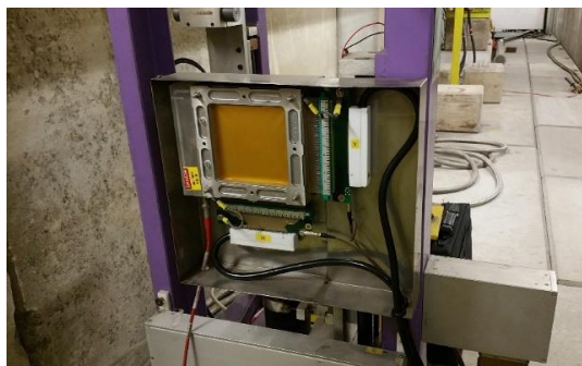
Fig. 4-35: A multi-wire proportional chamber in the North Area (XWCA 021 492).
