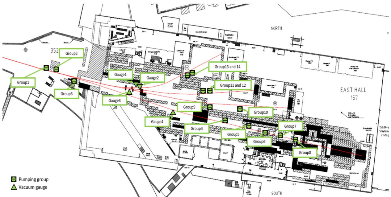
Fig. 4-17: Layout of the new vacuum system
