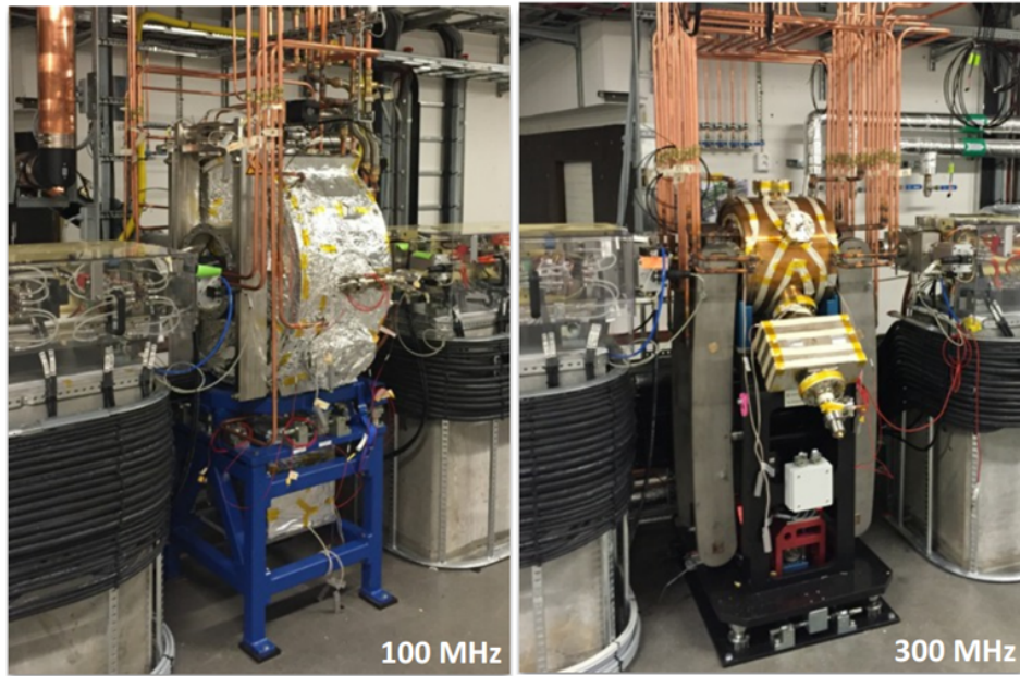
Fig. 10.6: A main cavity and the Landau cavity as installed in the MAX IV 3 GeV ring
