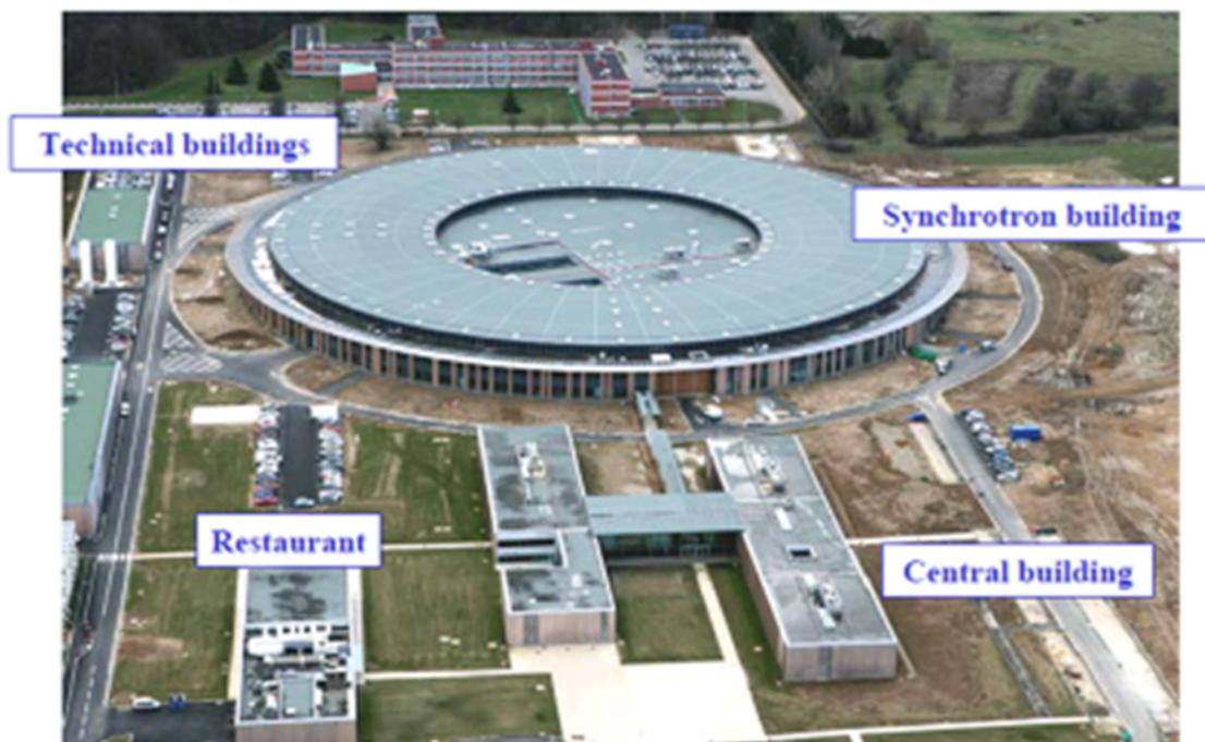
Fig. 16.9: Aerial view of the SOLEIL site, showing the spaces for the building, infrastructure, offices, parking, etc.
