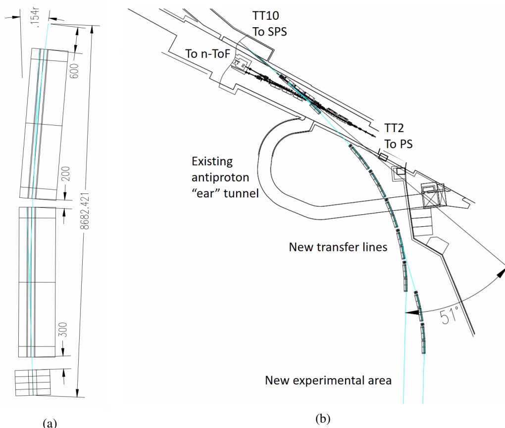
Figure 4.12: Schematic view of the base cell used in the new line with important dimensions in mm or rad (a) and layout of the new line in the junction region (b), with electron trajectory in cyan.
