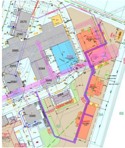
Figure 15-9: The LHC Point 5 with the new HL-LHC surface buildings in orange. Simple concrete slabs are highlighted in yellow.
