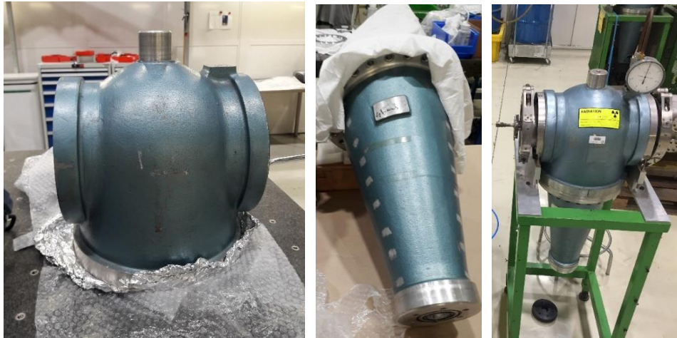
Fig. 4-31: New Cherenkov counter. Left: body; centre: conical part; right: complete assembly.
