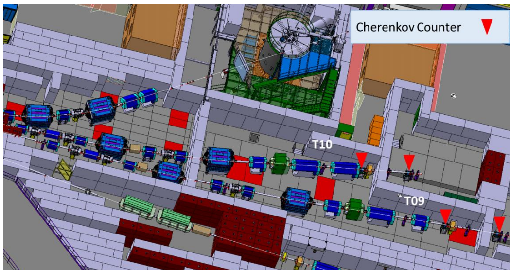
Fig. 4-30: Location of the new Cherenkov counters in the T09 and T10 beamlines.
