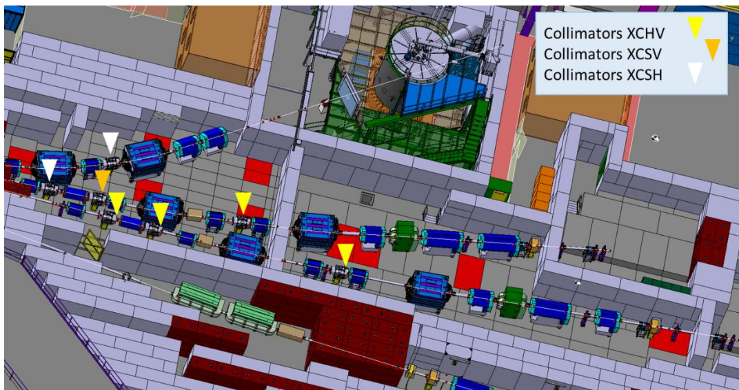
Fig. 4-42: Location of the new collimators in T09, T10 and T11.
