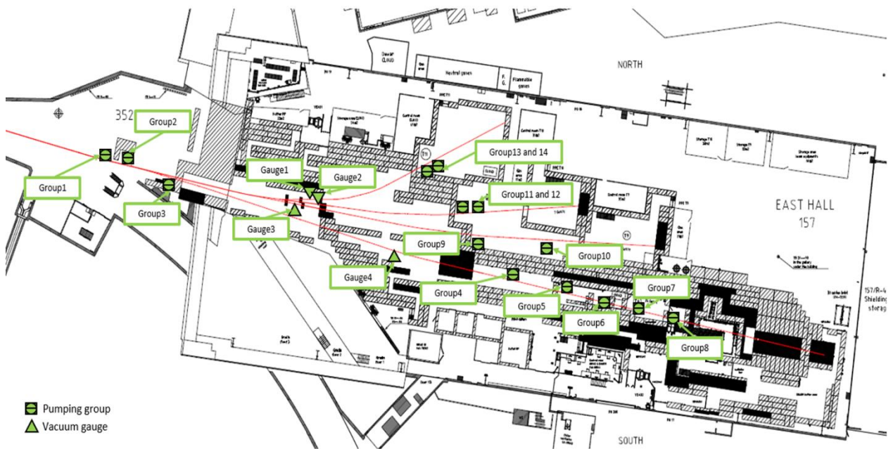
Fig. 4-17: Layout of the new vacuum system
