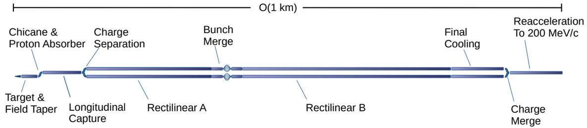
**Fig. 5.2:** Schematic of the muon production system. Protons are incident onto the target on the left of the figure, while the cooled muon beam leaves on the right of the figure, entering into the low energy acceleration system
