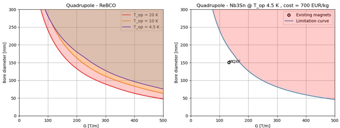
**Fig. 6.5:** Limitation curves as a function of stress and margin shown against bore diameter vs. magnetic field gradient of collider quadrupoles consisting of ReBCO at different operating temperatures (left) or Nb<sub>3</sub>Sn at 4.5 K (right). This is a current work in progress, with final design targets still being decided and protection limits created. Plots courtesy of D. Novelli.
