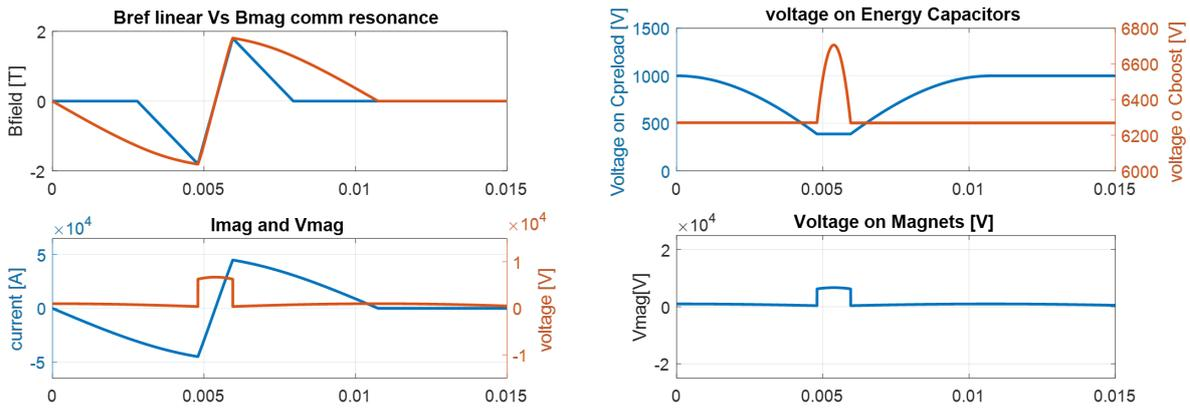
Fig. 6.10: Simulation of a switched resonance case
