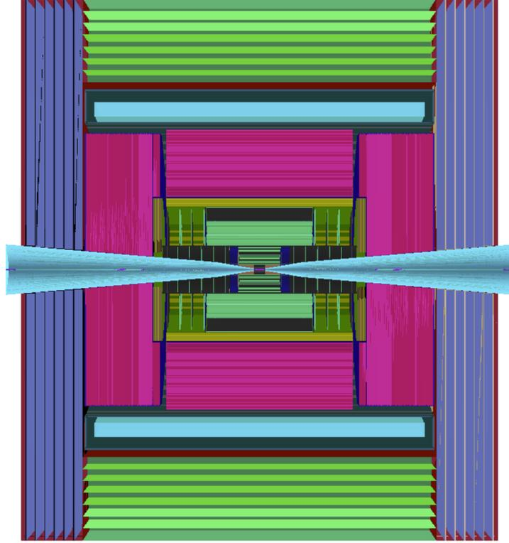
**Fig. 4.1:** Muon collider detector concept. From the innermost to the outermost regions, it includes the nozzles (cyan), the tracking system (light green), the electromagnetic calorimeter (yellow green), the hadronic calorimeter (red), the superconducting solenoid (light blue), and muon detectors (light green and blue).
