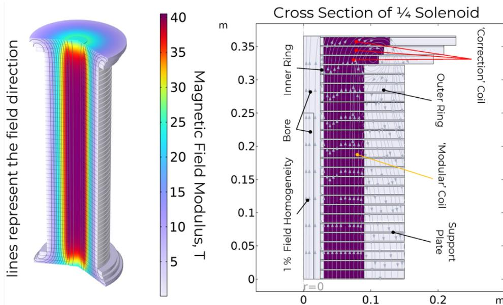
**Fig. 6.3:** The current 40 T and beyond conceptual design for the final cooling solenoids. It consists of 46 identical 'modular' and six 'correction' pancakes, with a bore aperture of 50 mm. Figures courtesy of B. Bordini.
