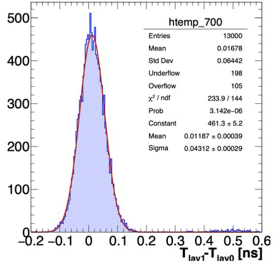
**Fig. 4.10:** Left: two out of three detection layers of the Crilin prototype proposed for Muon Collider calorimeter tested at CERN test beam. Right: Distribution of the time difference between two neighbouring layers of the prototype measured obtained with test beam data.
