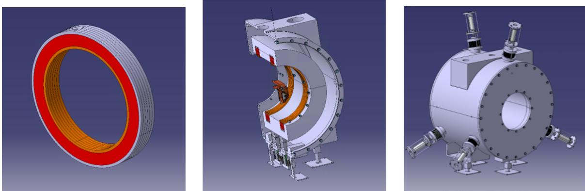
**Fig. 8.7:** Left. Single HTS coil with its restraining ring. Center: view of longitudinal cut of the spit coil system with inside the 3 GHz RF cavity (without ancillary systems). Right: the complete cryomagnetic assembly system for the 7 T RFMFTF.
