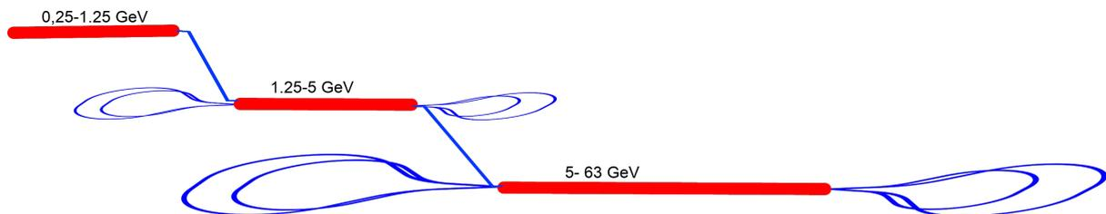
**Fig. 5.5:** Layout of a two-step-Dogbone RLA complex. Pre-accelerator, Dogbone I and Dogbone II are stacked up vertically;  $\mu^\pm$  beam can be transferred between the accelerator sections by the vertical dogleg.
