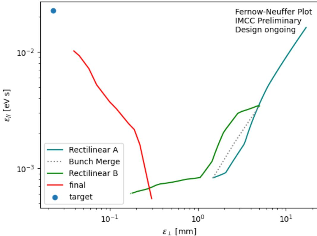
**Fig. 5.4:** System performance of the muon cooling system, including an updated rectilinear and final cooling system. Optimisation continues; in particular the rectilinear cooling system final emittance has not been integrated with the final cooling system.
