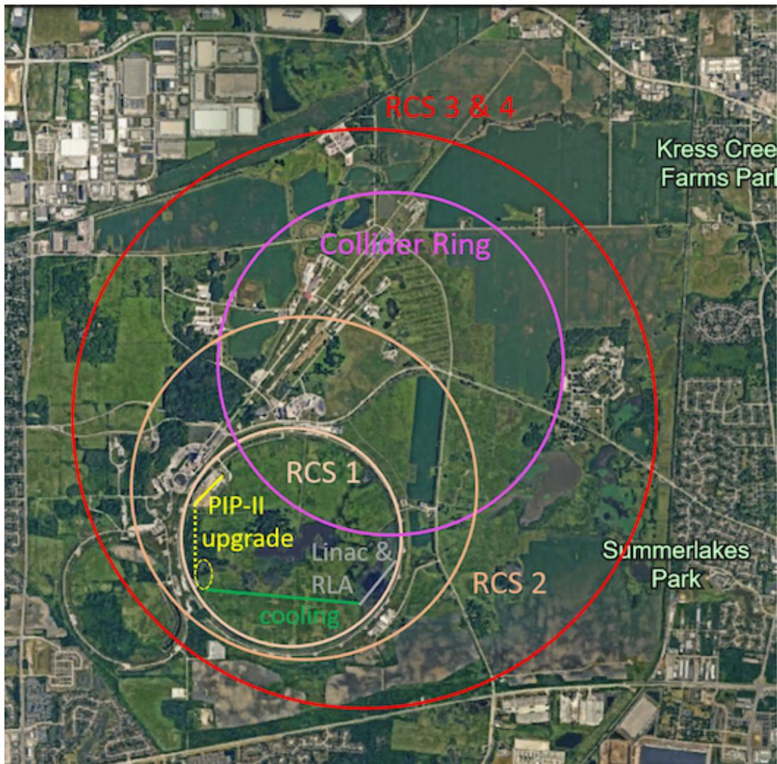
**Fig. 9.1:** Proposed layout of a 10 TeV center-of-mass energy muon collider complex sited at Fermilab. The proton driver is shown in blue and the cooling channel is shown in green. RCS1 can be located inside the existing Tevatron tunnel. RCS3 and RCS4 are located inside the Accelerator Ring with circumference of 16.5 km, which is the largest we can fit onsite.
