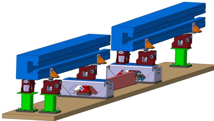
**Fig. 6.22:** Mock-up of the proposed magnet movement system.
