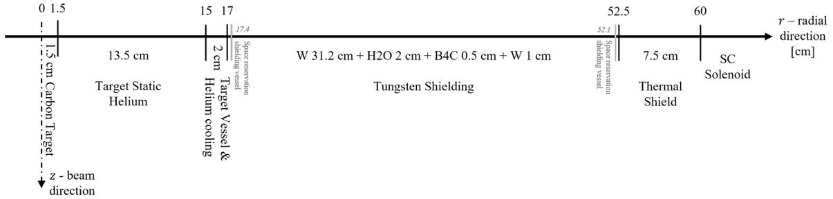
**Fig. 5.3:** Target assembly radial build showing different azimuthal regions from the target the axis up to the SC solenoid coils.
