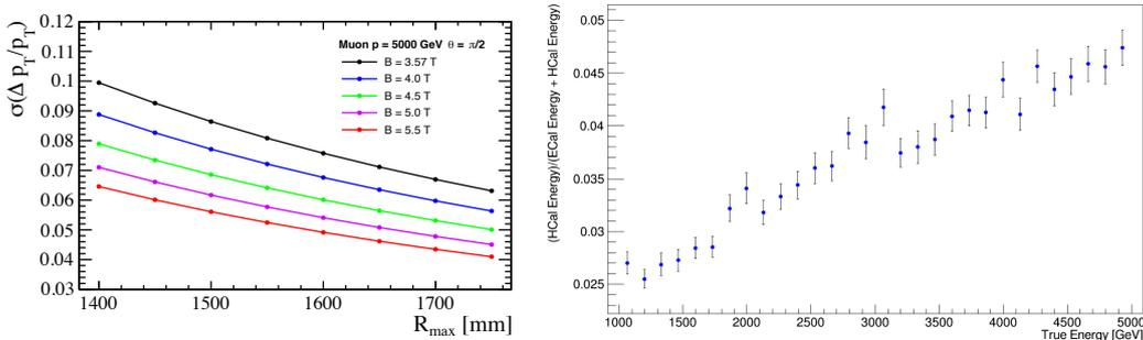
**Fig. 4.4:** Left: track momentum resolution for muons with  $p = 5$  TeV and  $\theta = \pi/2$ , as a function of the tracker radius ( $R_{max}$ ) and for different values of magnetic field ( $B$ ). Right: fraction of photon energy measured in HCAL with respect to the total energy measured in ECAL+HCAL, as a function of the true photon energy.
