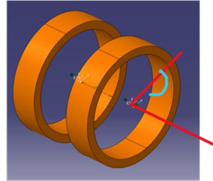
**Fig. 8.5:** Sketch of the RFMFTF with an RF cavity inside the magnet bore.
