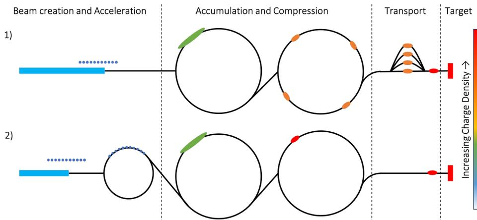
**Fig. 5.1:** Schematic layouts for the proton complex section. Our baseline design is the schematic 1 on the figure. The bunch density as the proton travels through the complex is also depicted. The closer to the target the highest the bunch charge density and at the point where it collides with the target. To reach high densities is one of the main challenges in the design of the part of the muon collider.
