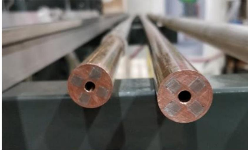
**Fig. 6.1:** MIT VIPER cable, image taken from Ref. [9].
