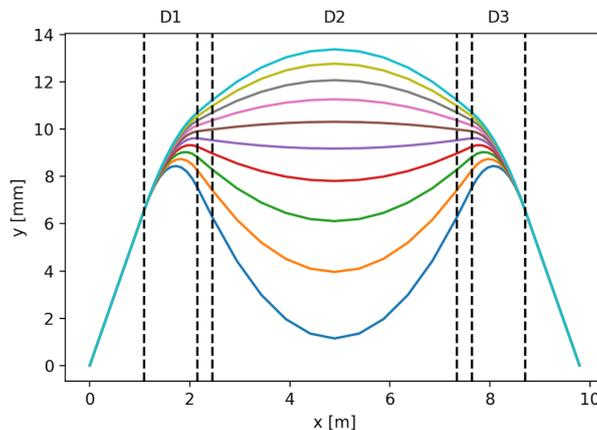
**Fig. 5.8:** Trajectories in a half-cell of RCS2. The injection/extraction orbits are respectively in the inner/outer side (in blue/cyan). From Ref. [7].
