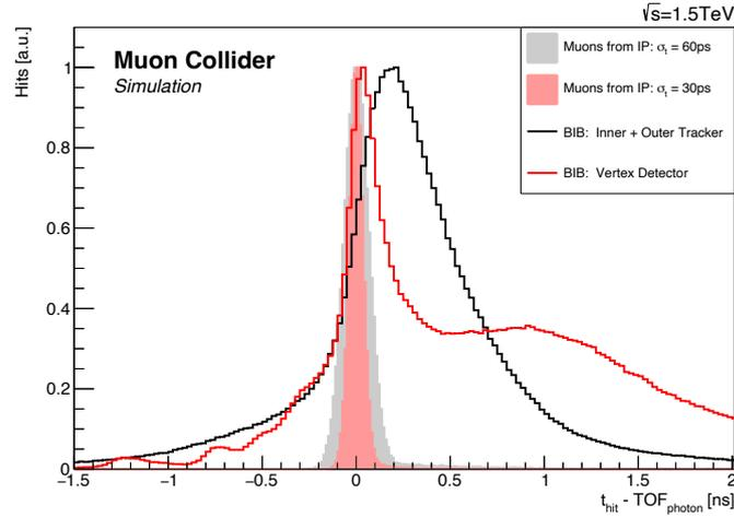
**Fig. 4.8:** Time distribution of hits in the tracking detector corrected for the expected photon's time of flight from the interaction point. Hits from the beam-induced background (BIB) are shown by solid lines, while hits from single muons smeared by corresponding time resolutions are shown by filled areas.
