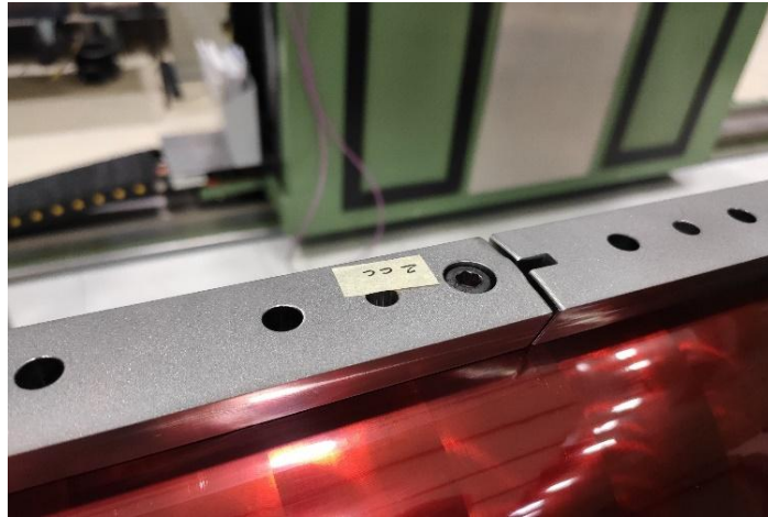
Figure 130: Layout of segmented Ti-alloy pole pieces in preparation for the winding of the inner layer of a 7.2-m-long HL-LHC MQXFB quadrupole magnet coil at CERN. The gap intentionally left between pole pieces is clearly visible at the picture center (Courtesy of N. Lusa, CERN, 2022).
