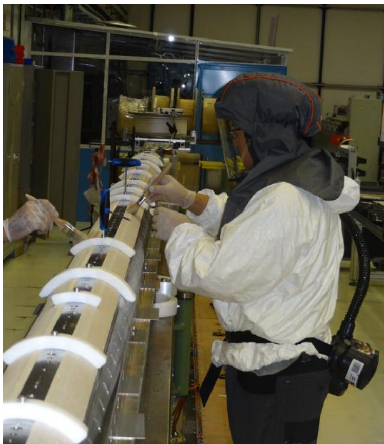
Figure 125: Application of ceramic binder on the outer surface of a wound 7.2-m-long HL-LHC MQXFB coil at CERN. The operation requires the use of personal protection equipment due to health and safety reasons (Courtesy of R. Berthet, FOSELEV, and R. Principe, CERN).
