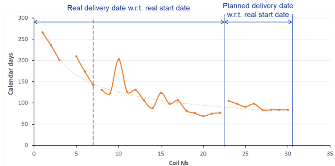
Figure 66: Duration of manufacturing process versus sequential number for 5.3-m-long, HL-LHC 11 T dipole magnet coil production by industrial supplier on CERN premises; data rely on expected delivery dates for last part of production to remove COVID-19 bias (Courtesy of F. Savary, CERN).
