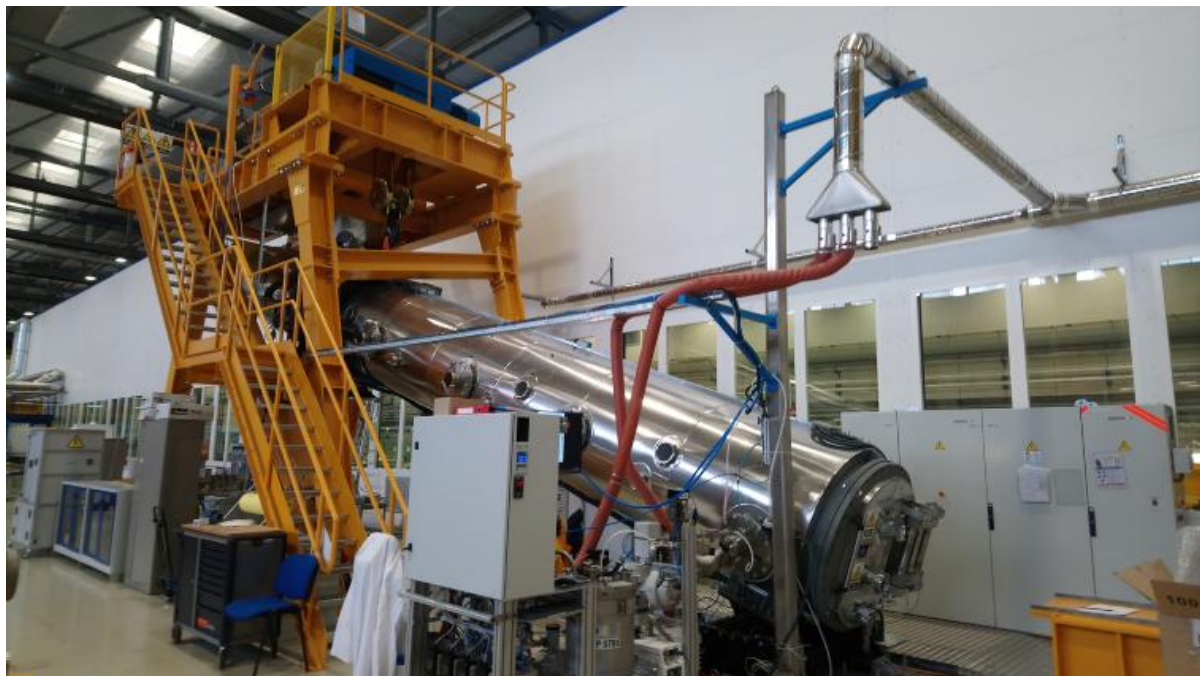
Figure 135: View of VPI station at CERN with vacuum tank tilted at 18° before start of resin impregnation (Courtesy of J. Axensalva, CERN).
