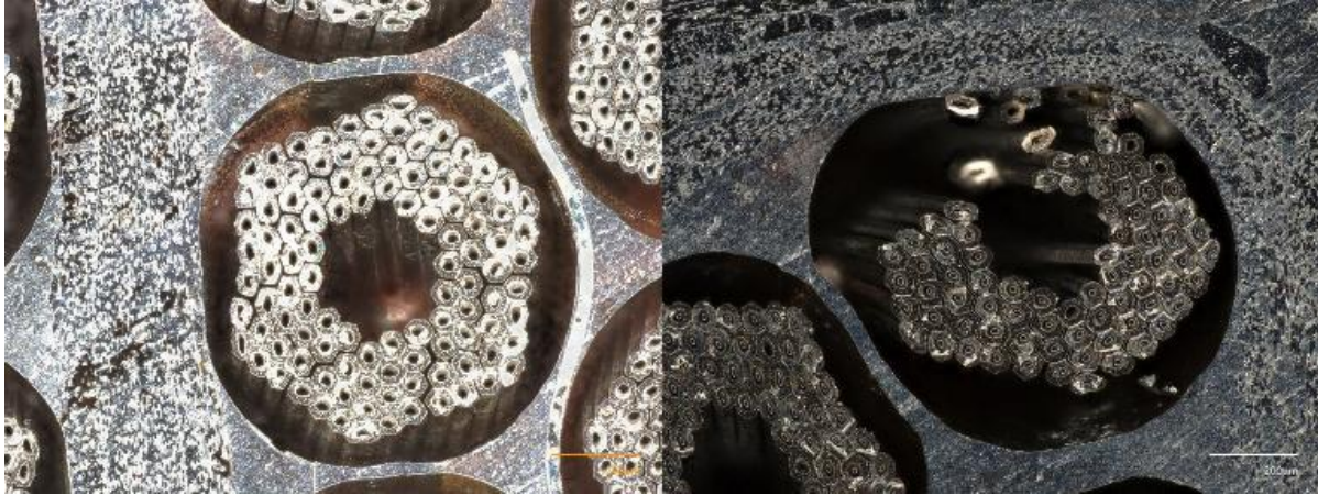
Figure 55: Optical images of resin-impregnated RRP® strands from transverse cross-sections of MQXF BP1 coil Q108 having been submitted to deep copper etching. Left: strand showing no degradation. Right: strand showing a number of broken tubular Nb 3 Sn sub-elements (courtesy of M. Crouvizier, CERN).
