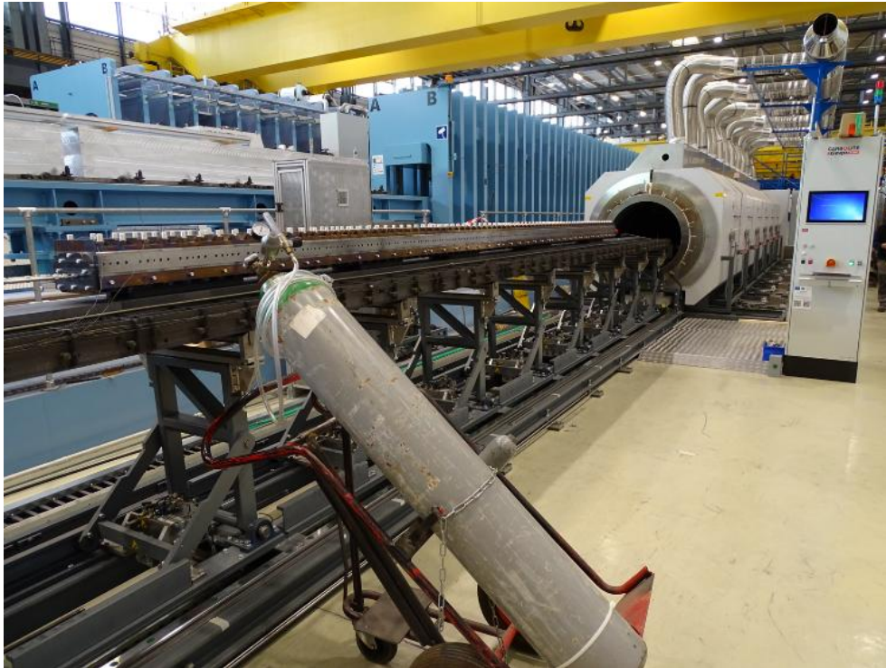
Figure 129: 7.2-m-long HL-LHC MQXFB quadrupole magnet coil in its retort ready for loading into heat treatment furnace. The foreground features a bottle of pure argon that will be connected to enable a flow through the coil (Courtesy of O. Housiaux, SERCO, and R. Principe, CERN).
