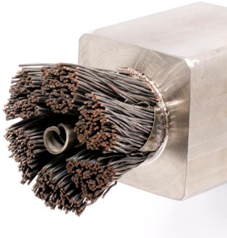
Figure 3: Photograph of a reacted ITER CS Cable-in-Conduit Conductor after partial removal of the austenitic steel, circle-in-square jacket and of the stainless-steel wraps around the 6 petals of the rope-type cable. The cable is manufactured in 5 stages and is made up of 576 Cr-plated Nb 3 Sn strands, mixed with 276 pure Cu strands, arranged around a central, austenitic steel, cooling spiral (courtesy of C. Sanabria, formerly ASC, 2013).
