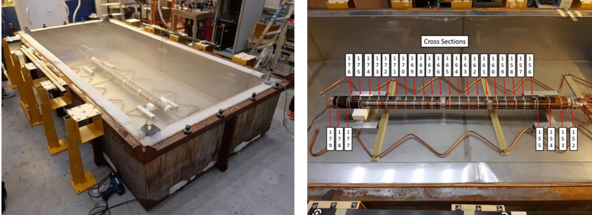
Figure 90: Experimental set up at CERN Cryogenic Laboratory to measure geometry changes on 2-m-long, HL-LHC 11 T dipole magnet coil SD122 between room and GN 2 temperature. Left: picture of coil in metallic container with plexiglass lid. Right: picture showing the position of the photogrammetric targets on the coil surface (Courtesy of J. Bremer, T. Koettig, and D. Mergelkuhl, CERN [247]).
