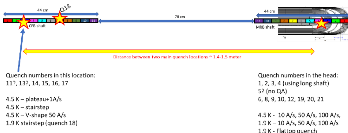
Figure 21: Quench-start localizations assessed on 5.3-m-long, series production, HL-LHC 11 T dipole magnet S4, showing the impact of the type of current ramps (Courtesy of G. Willering, CERN).
