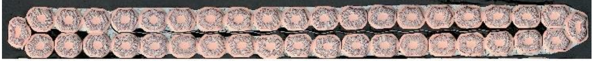
Figure 6: Cross-sectional view of an un-reacted MQXFB Rutherford-type, cable made up of 40 Nb 3 Sn RRP® strands and a 25- \mu m-thick, 12-mm-wide stainless-steel core between the strand layers. The cable has a slight keystone angle of 0.42° (the thin edge is on the right side of the picture). The grey zones between strands correspond to the resin used for potting the cable sample for metallographic purposes (Courtesy of A. Bonasia, CERN).
