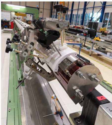
Figure 124: Clamping tools used during the winding of 7.2-m-long HL-LHC MQXFB quadrupole magnet coil ends at CERN (Courtesy of R. Berthet, FOSELEV, and R. Principe, CERN).
