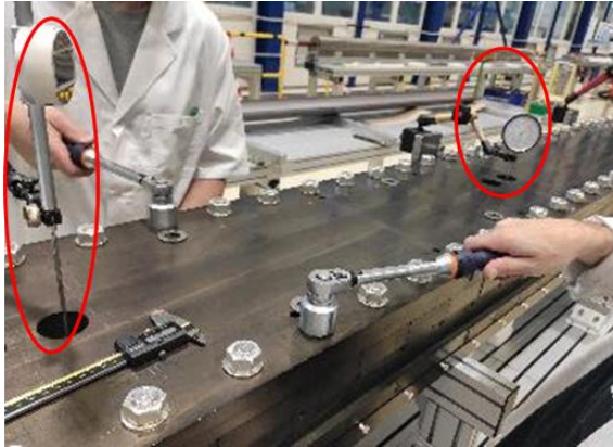
Figure 131: Dial gauge measurements carried out at various steps of retort opening after reaction heat treatment of 7.2-m-long HL-LHC MQXFB quadrupole magnet at CERN. Left: coil vertical displacement measurements. Right: coil elongation measurements. The largest displacements/elongations occur at the time of unbolting of M20 screws (Courtesy of N. Lusa, CERN).
