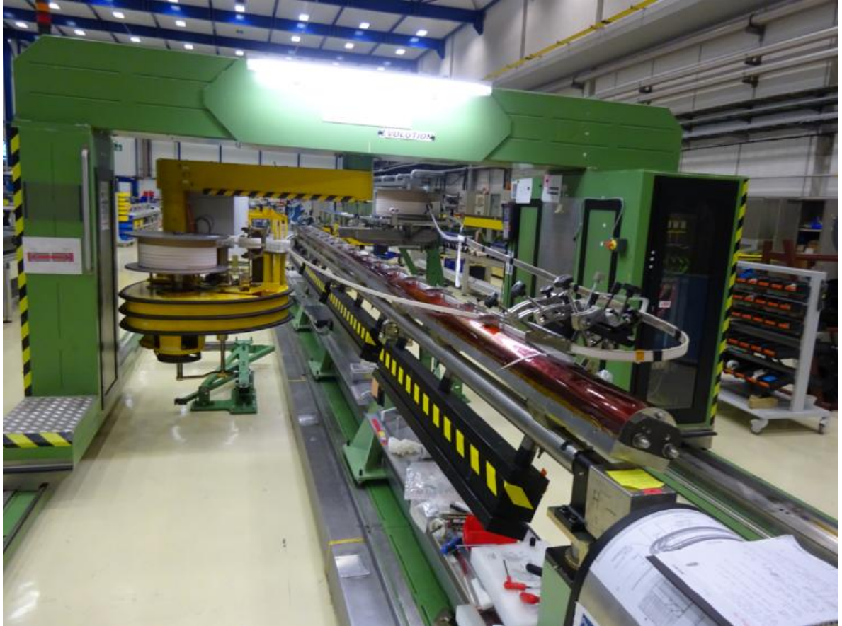
Figure 123: Winding of a 7.2-m-long HL-LHC MQXFB quadrupole magnet coil at CERN (Courtesy of R. Berthet, FOSELEV, and R. Principe, CERN).
