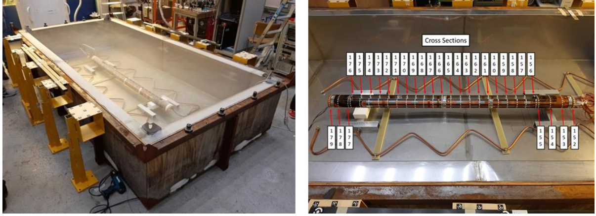
Figure 90: Experimental set up at CERN Cryogenic Laboratory to measure geometry changes on 2-m-long, HL-LHC 11 T dipole magnet coil SD122 between room and \text{GN}_2 temperature. Left: picture of coil in metallic container with plexiglass lid. Right: picture showing the position of the photogrammetric targets on the coil surface (Courtesy of J. Bremer, T. Koettig, and D. Mergelkuhl, CERN [247]).
