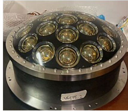
Fig. 6-6: A multi-PMT photodetector system for the Hyper-Kamiokande experiment.
