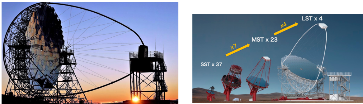
Fig. 35-3: Picture from a CTA LST operational in La Palma since 2020. LST (diameter = 23 m): mirror area of 400 m² (left) and size comparison of the CTA telescopes (right).
