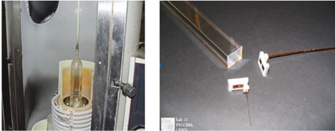
Fig. 23-9: CMS crystal. Drawing a crystal of lead-tungstate (left). The avalanche photodiodes for its read-out used in CMS (right) 632 .
