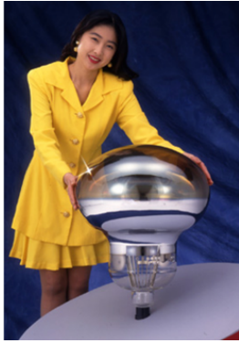
Fig. 6-5: Picture of a very large PMT used in the Kamiokande \nu physics experiment (Japan).
