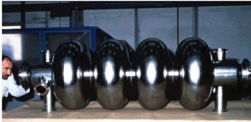
Fig. 15-8: LEP SC RF cavity.
