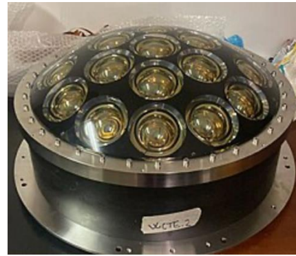
Fig. 6-6: A multi-PMT photodetector system used in the Hyper-Kamiokande experiment.
