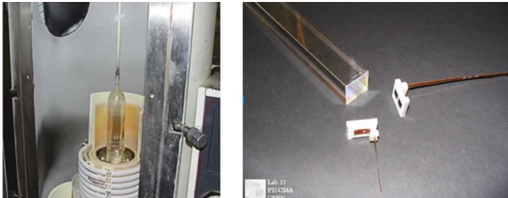
Fig. 23-9: CMS crystal. Drawing a crystal of lead-tungstate (left). The avalanche photodiodes for its read-out used in CMS (right) 670 .
