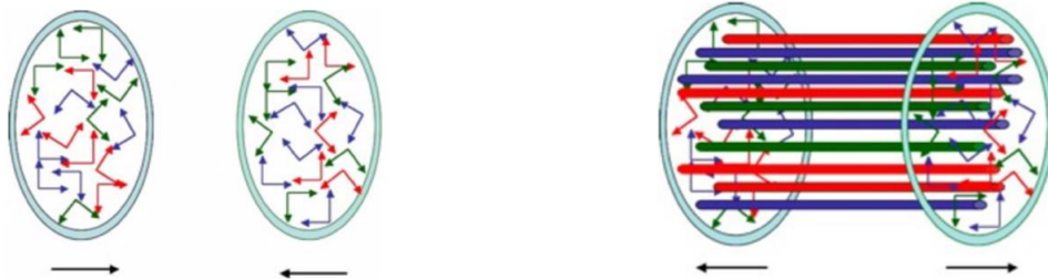
Fig. 20-18: Left: classical fields, prior to the collision, are transverse to the direction of motion. Right: longitudinal colour electric and colour magnetic fields between the sheets 629 .
