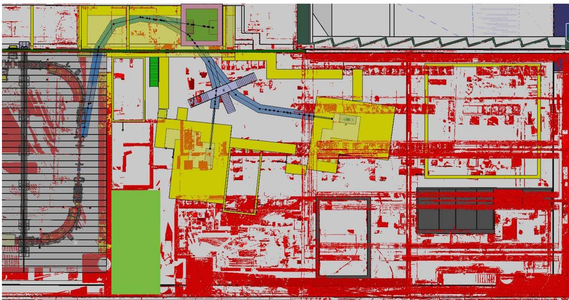
**Fig. 12.1:** A 3D scan of hall 150, in red, shows mostly stored material. The loading dock zone for the crane is indicated in green and the Research and Development areas (XBOX and EBIS) are shown in grey. The layout of the new experimental area for the BioLEIR facility is superimposed in yellow.
